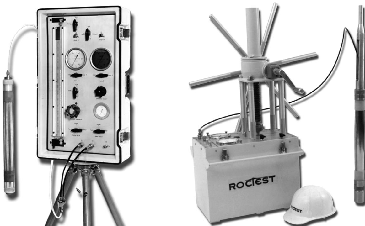
Figure 5. G-AM and TEXAM pressuremeter models
