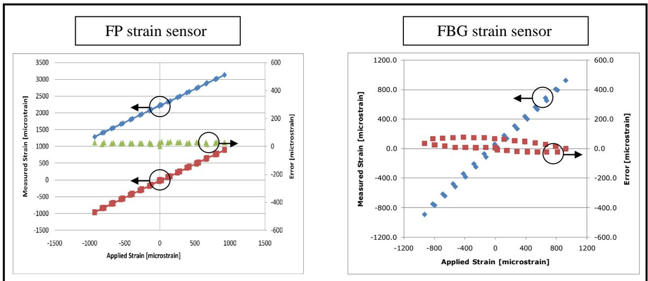
Figure 7. Strain accuracy test results at nitrogen temperature.
