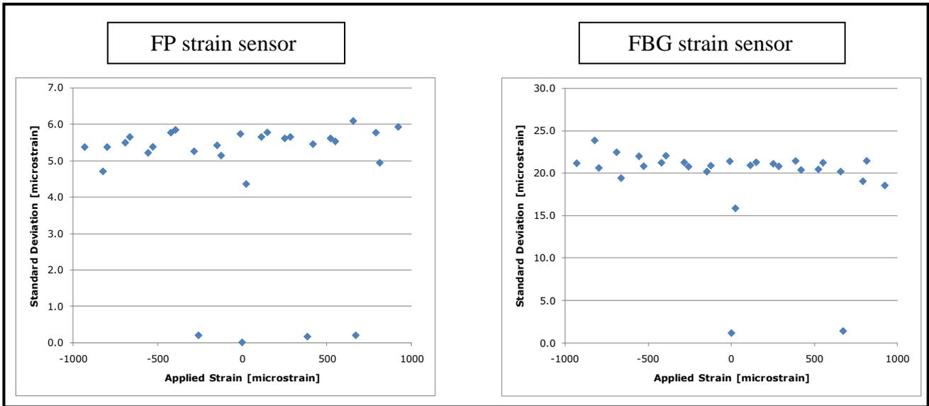
Figure 6. Strain resolution test results at nitrogen temperature.
