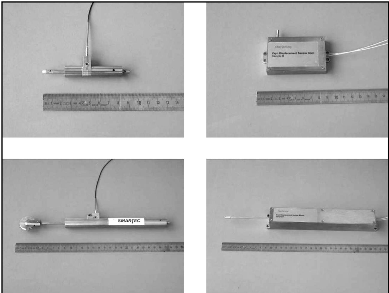
Figure 8. Fibre Optic displacement sensors, FP small displacement top left, FBG small displacement top right, FP large displacement bottom left, FBG large displacement bottom right
