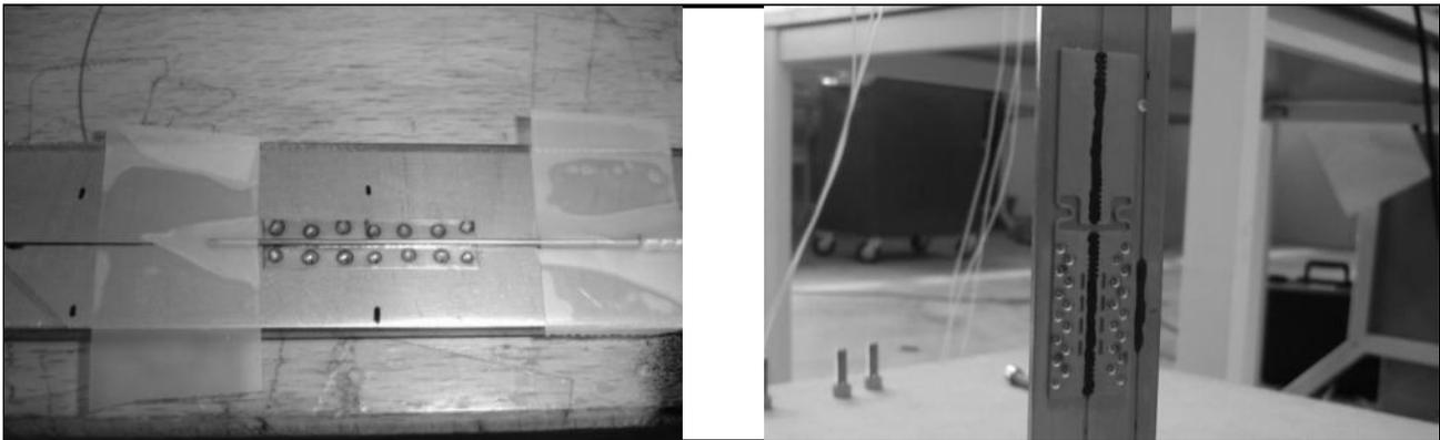
Figure 5. Fibre Optical strain sensors, FP left, FBG right, during testing.
