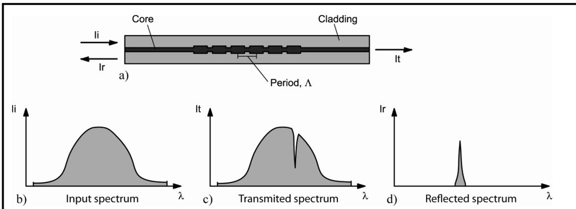
Figure 3. Functional principle of Fibre Bragg Grating sensors.
