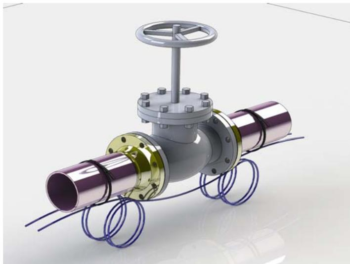
**Figure 9:** *Installation on valves.*
