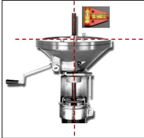
**Importance of carefully aligning the recording unit with the borehole casing (auger) and the rods**
