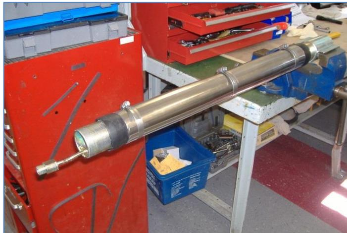
Figure shows a new membrane being assembled on the body of the probe.
