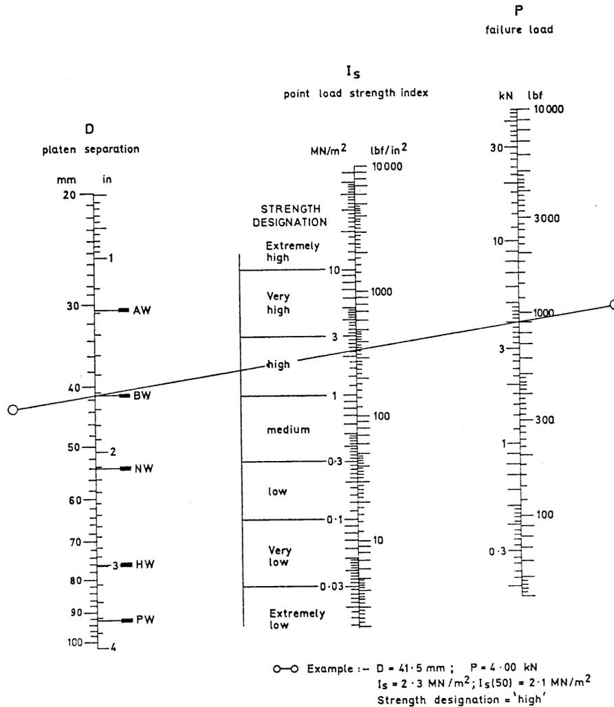
**Figure 2: Nomogram for computing point load strength**
