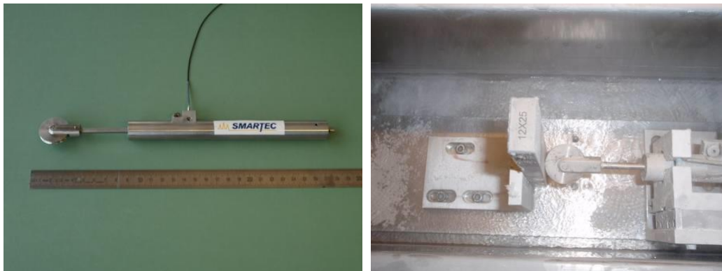
Figure 9. Fiber optic displacement sensor for ITER and cryogenic testing.
