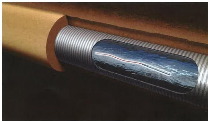
Figure 7. Compact fiber optic piezometer for dike monitoring.
