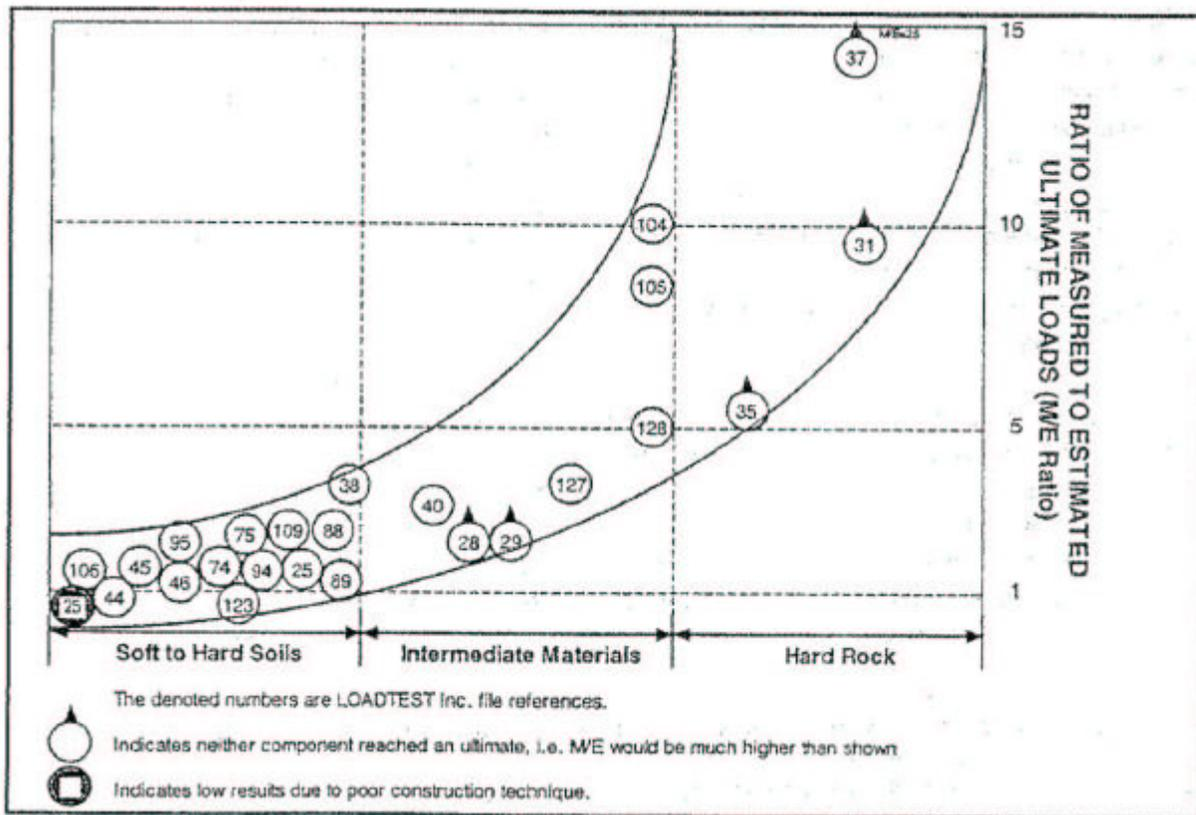
Figure 1. Underestimating rock capacity (Schmertmann and Hayes)
