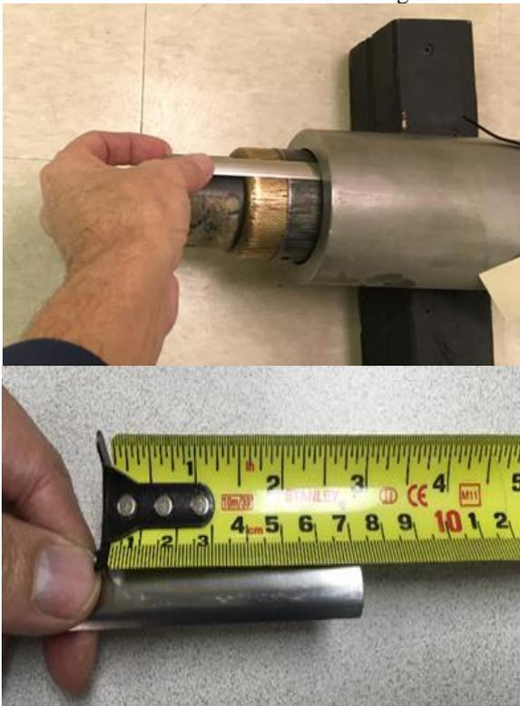
Figure 5. Measuring CL with a steel strip
