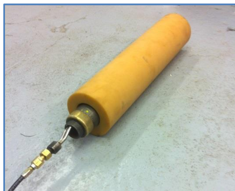
Figure 1. Pressuremeter Probe in the Polyurethane Tube
