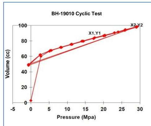
Figure 5. Test results showing elastic responses of rock masses (Courtesy: Fugro-Sial Ltd. from Turkey)
