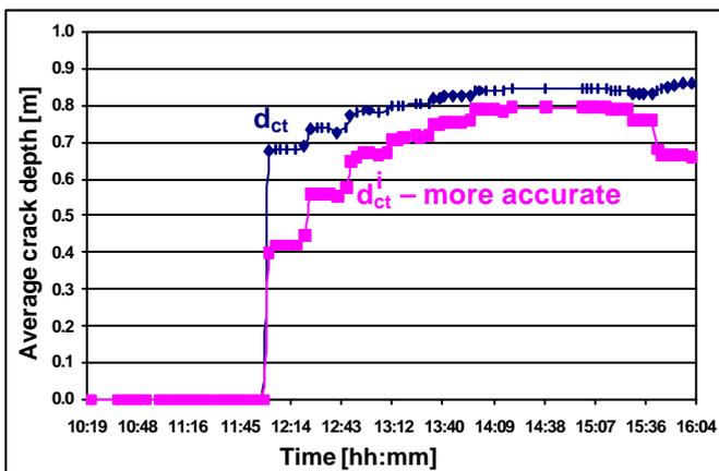
Figure 12. Evolution of average crack depth
