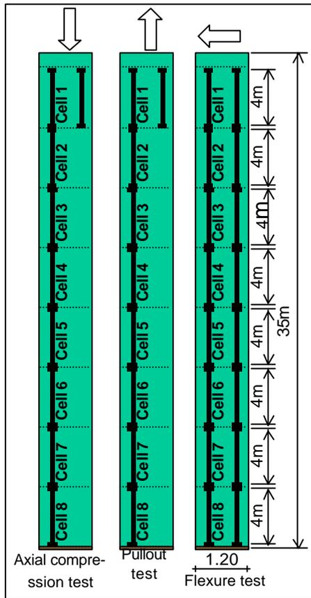
Figure 5: Topologies applied in piles monitoring and dimensions of piles.
