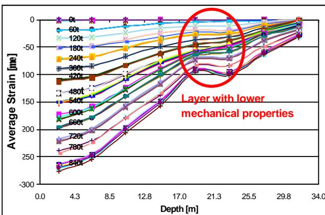
Figure 7. Average strain distribution, increase of load, axial compression test.
