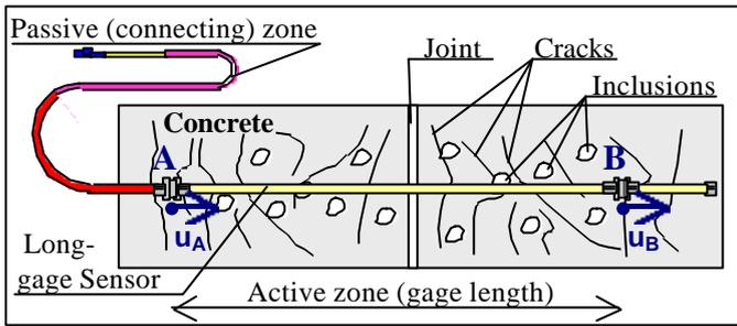
Figure 1: Schema of a long-gage sensor installed on a material with cracks, inclusions and joints.
