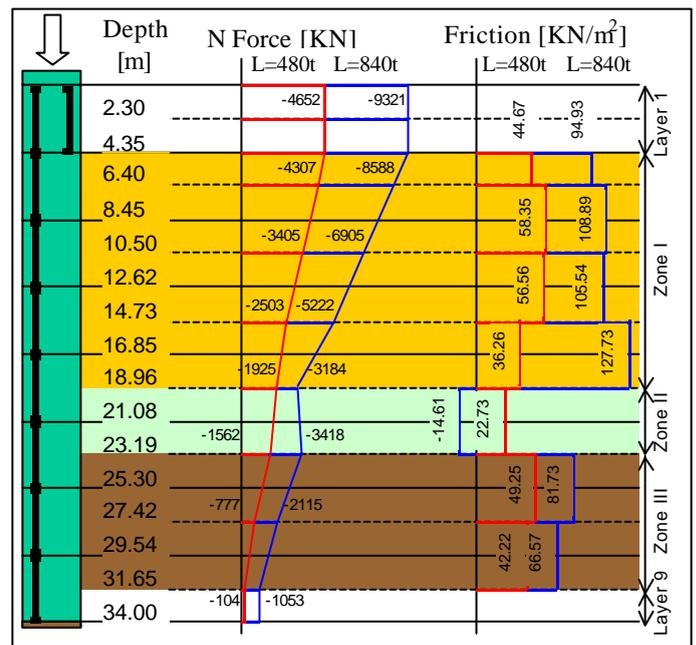
Figure 9. Distributions of normal force in the pile, friction stress and different zones of soil, axial compression test.
