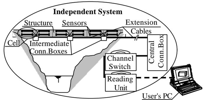
Figure 2: Schema of a structure divided in cells with parallel topologies of long-gage fiber optic sensors of type SOFO.
