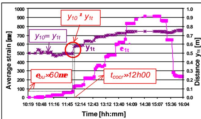
Figure 11. Determination of crack occurring time and ultimate strain of concrete.
