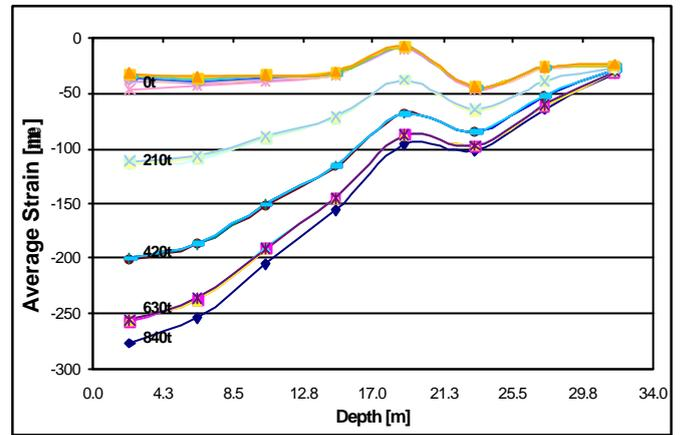
Figure 8. Average strain distribution, unloading, axial compression test.
