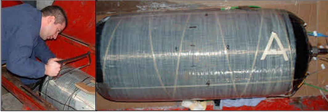
Fig. 10: Damaging of tank "A" (cuts) and view to damaged tank
