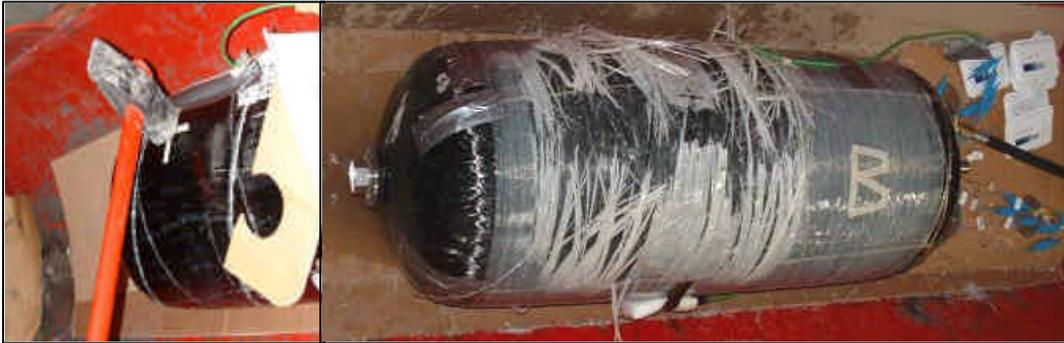
Fig. 11: Damaging of tank "B" (shocks) and view to damaged tank after burst
