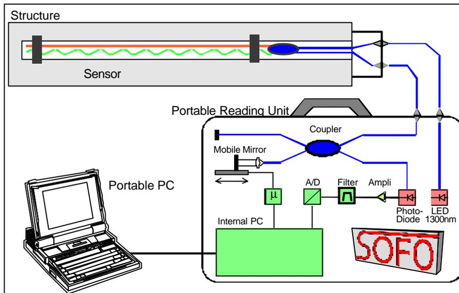
Fig.3: Components and functional principle of the SOFO system
