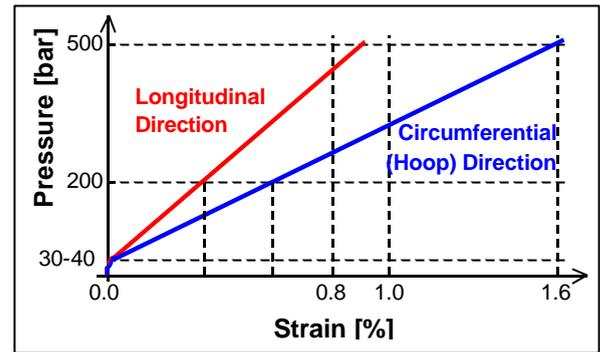
Fig. 2: Expected strain-pressure diagram of tank
