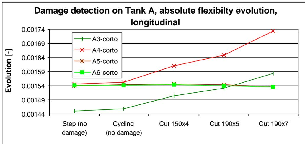
Fig. 14: Increase of absolute flexibility coefficients indicates the damage between sensors A3 and A4 (see Fig. 10)
