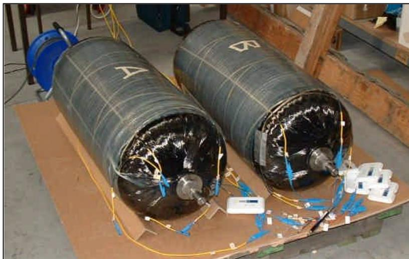
Fig. 6: View to full composite tanks with embedded SMARTapes and connection boxes
