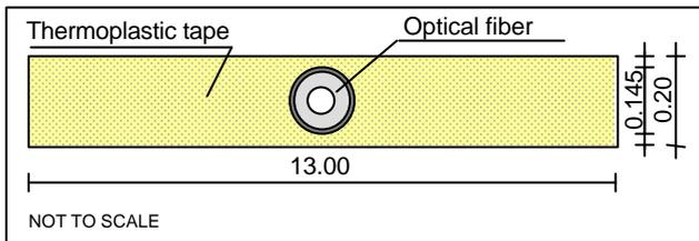
Fig. 4: Typical cross-section of SMARTape
