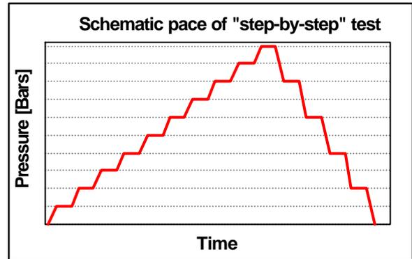
Fig. 9: Schematic representation of step-by-step test pattern
