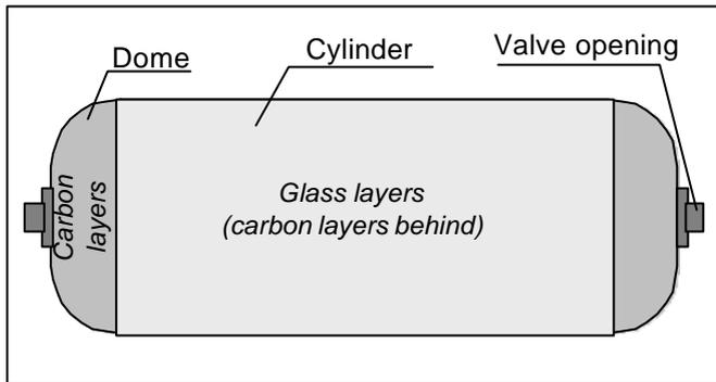
Fig. 1: Schematic representation of tank and its components
