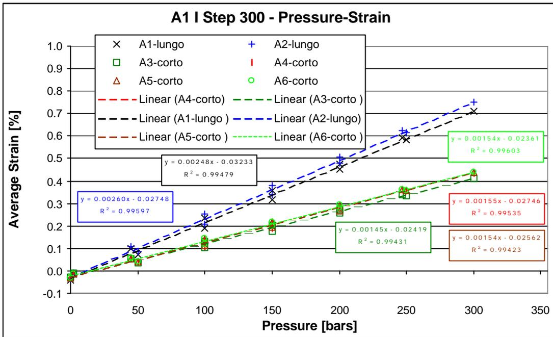
Fig. 12: Example of typical pressure-strain diagram of tanks
