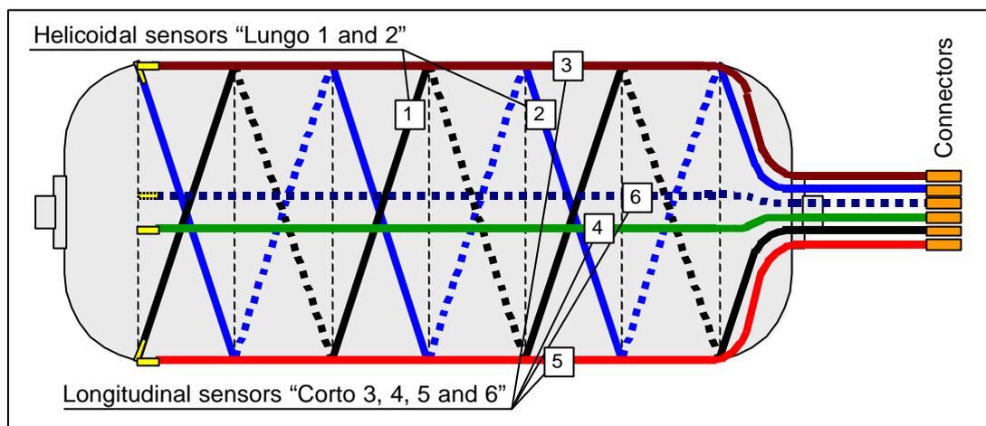
Fig. 7: Topology of sensors (SMARTapes) embedded in tank
