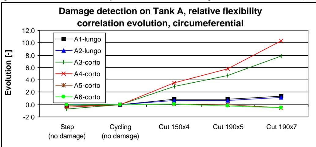
Fig. 15: Increase of absolute flexibility coefficients indicates the damage; hoop sensors are also slightly affected
