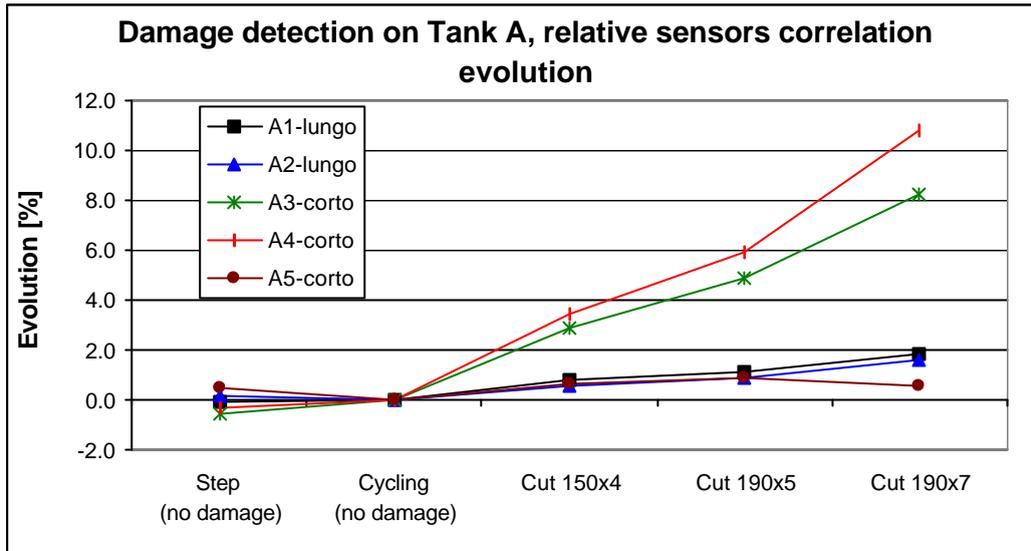
Fig. 16: Change (increase) of flexibility coefficients indicates the damage; separation of lines indicates damage too
