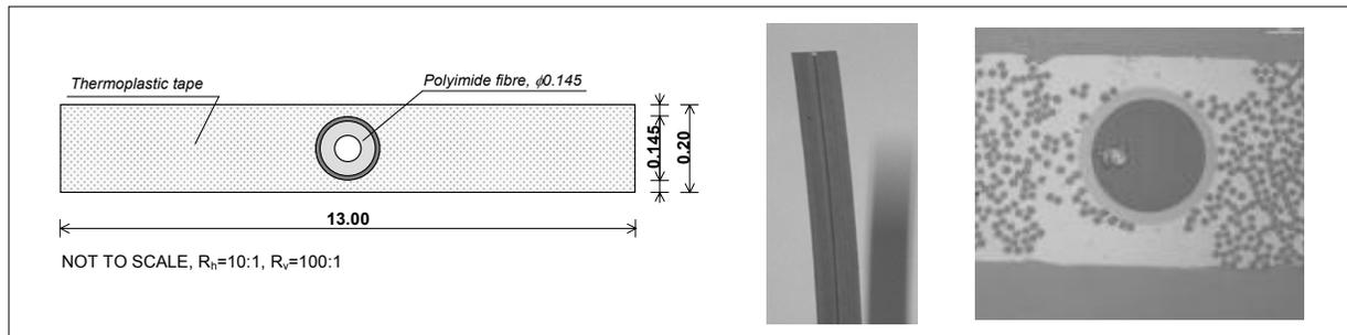
Fig. 3. Cross-section picture and micrograph of the sensing tape: SMARTape.
