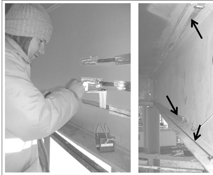
Fig. 5. On-site test of SMARTape gluing procedure (left) and installed SMARTapes for full performance tests (right).
