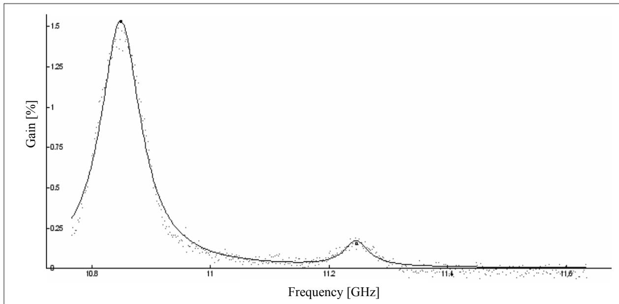
Fig. 4. Main Brillouin peak generated by strain variation over spatial resolution length, and secondary peak generated by crack.
