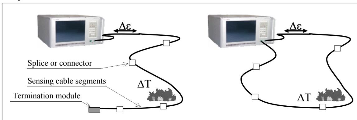
Fig. 2. Schemas of DiTeSt system configurations; left: single ended configuration; right: loop configuration.
