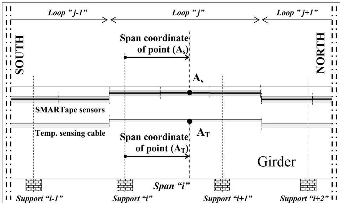
Fig. 8. General position of spans and loops.
