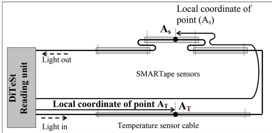
Fig. 7. Basic sensing loop consisting of three SMARTape sensor of 90 m and temperature sensing cable.
