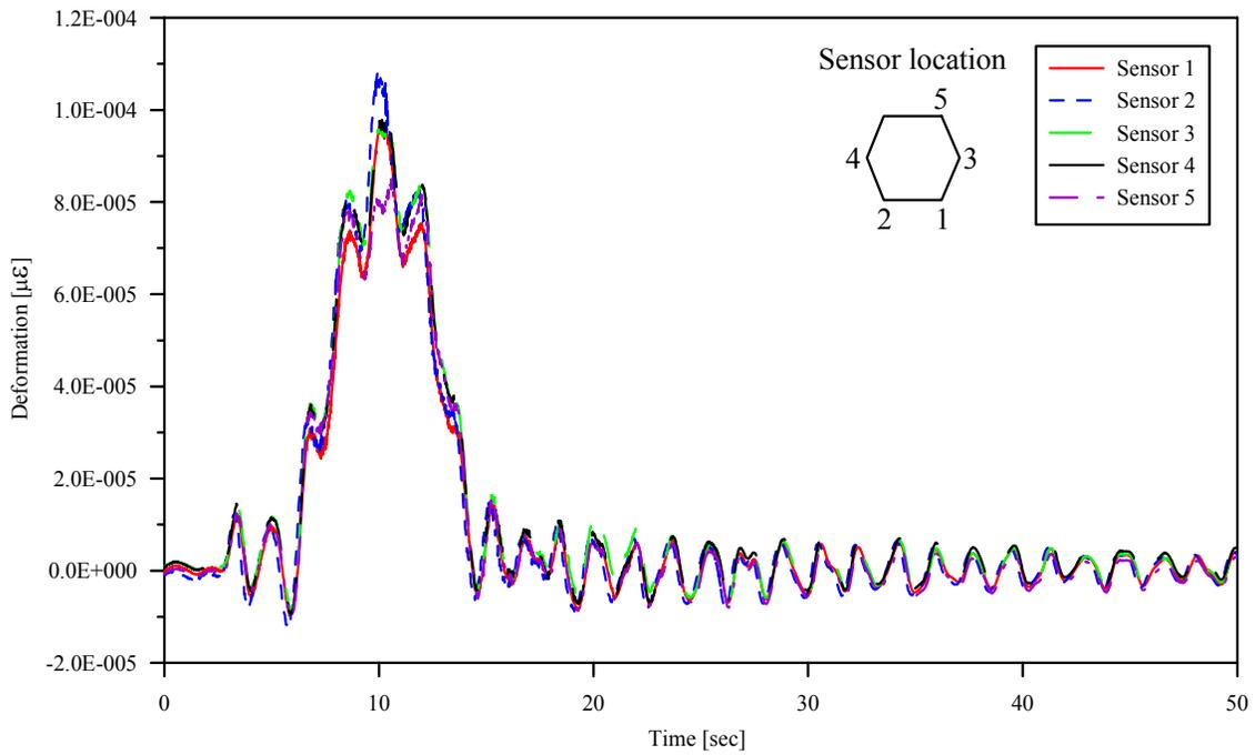
Figure 8. SOFO deformation sensor readings at the centre of the bridge for 2 trucks moving at 72 km/h.
