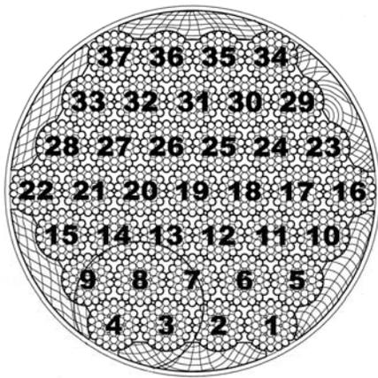
Figure 2. Typical cable section (37 strands, 1591 wires in total).
