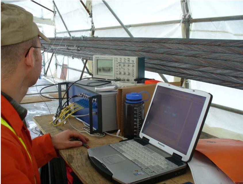
Figure 4. SOFO sensors, open cable section.
