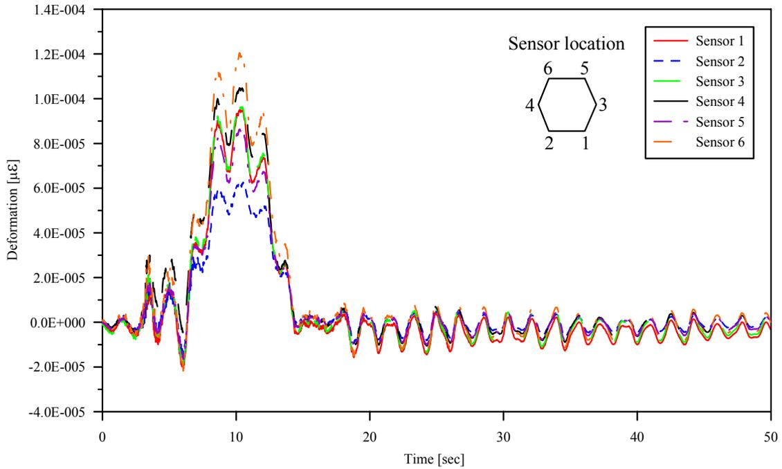
Figure 9. SOFO deformation sensor readings at the anchor block for 2 trucks moving at 72 km/h.
