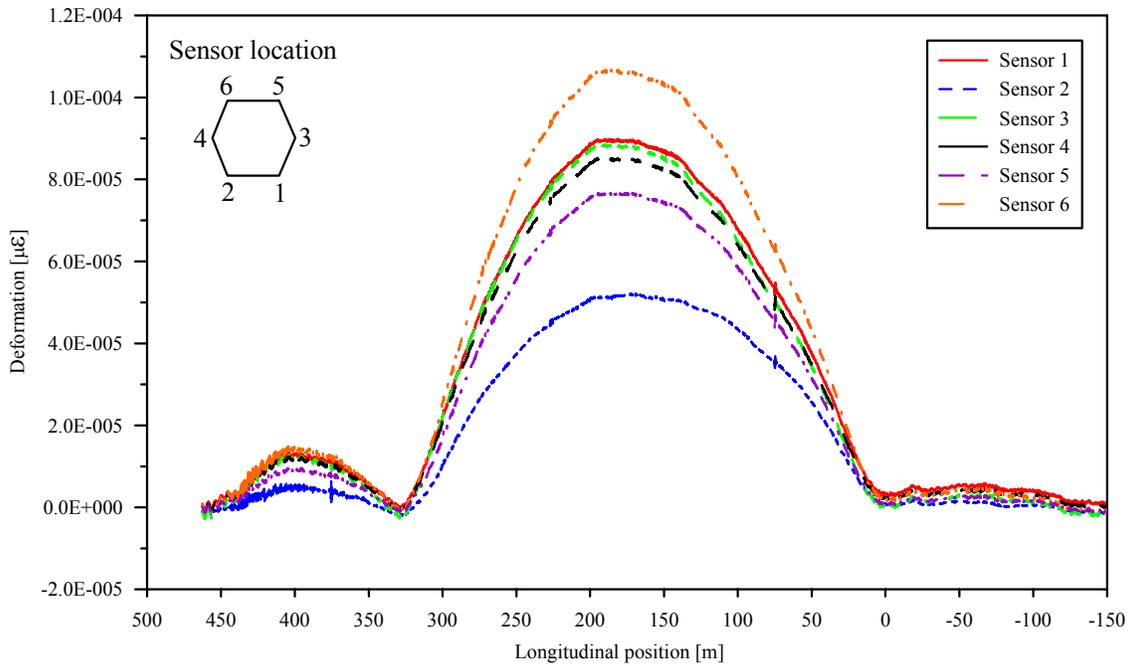
Figure 7. SOFO deformation sensor readings at the anchor block for 2 trucks moving at 7 km/h.
