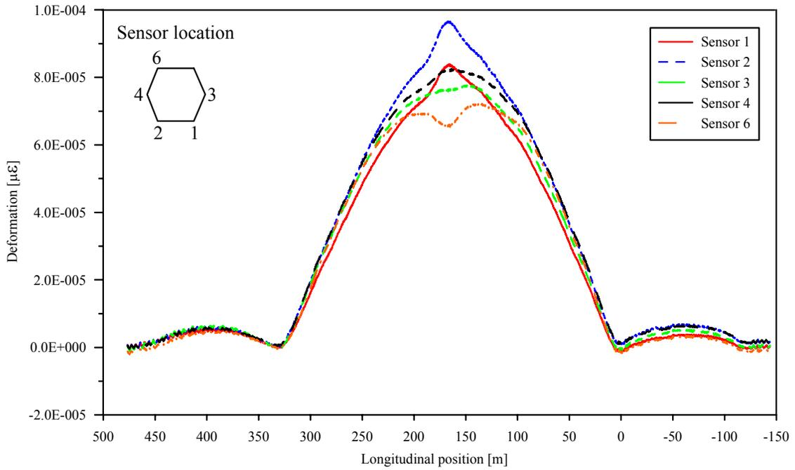
Figure 6. SOFO deformation sensor readings at the centre of the bridge for 2 trucks moving at 7 km/h.
