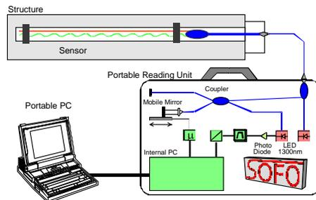
Figure 6. Setup of the SOFO system used for static measurements.
