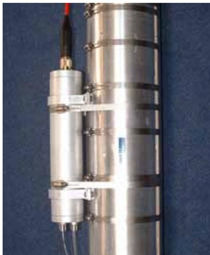
Figure 3. Watertight junction box with connector and optical cable.
