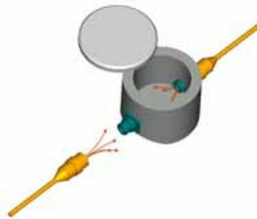
Figure 4. Alternate design of the underwater junction box. (Not included in the qualification project)
