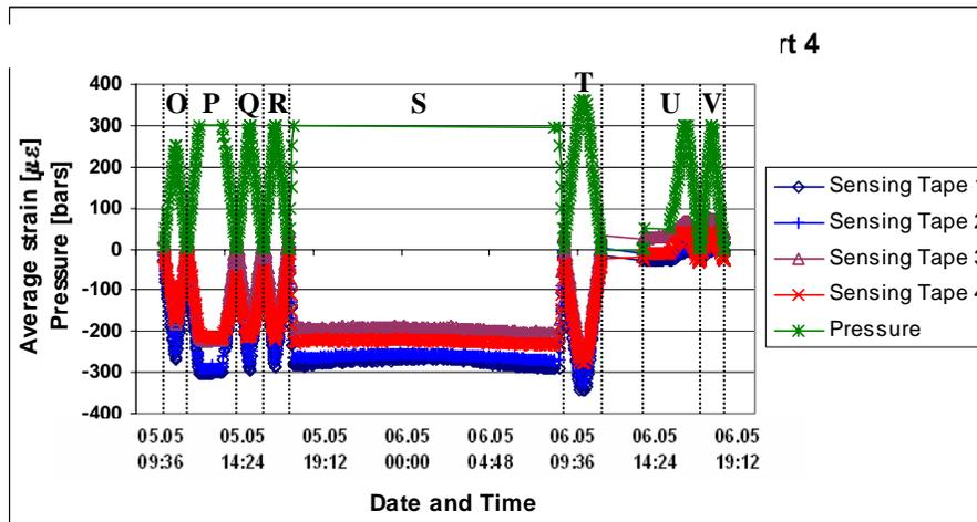
Figure 12. Hyperbaric chamber testing results: Pressure cycling with closed and open riser section.
