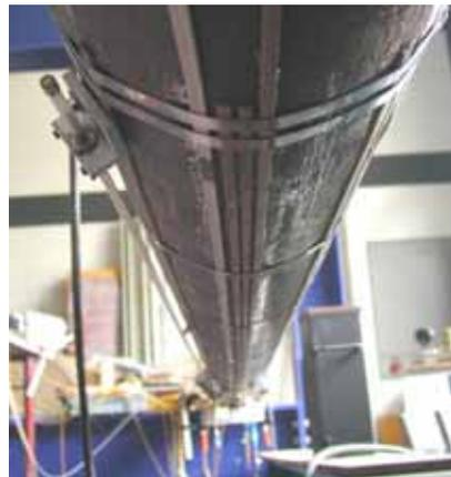
Figure 11. Detail of the installation of the sensors on the full-scale 6 m-long riser section.
