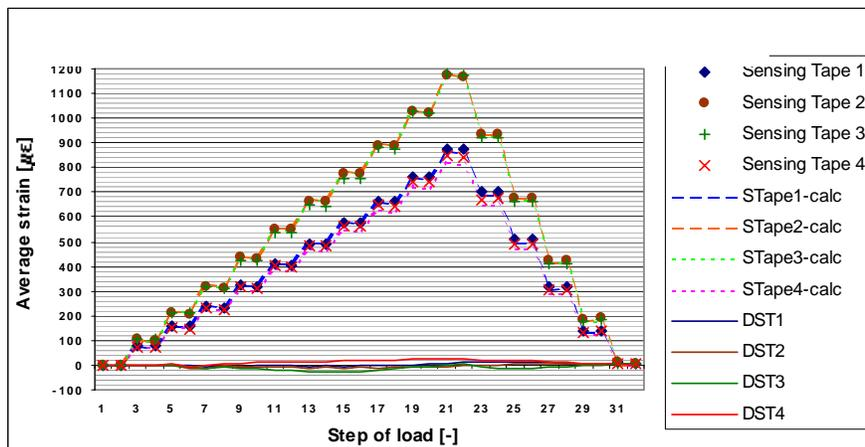
Figure 13. Full-scale testing results: Comparison of measured and theoretical strains and residual differences.
