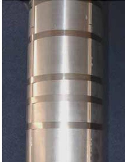
Figure 1. Sensors glued and clamped to a riser section.
