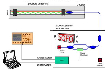
Figure 7. Setup of the SOFO system used for dynamic measurements.
