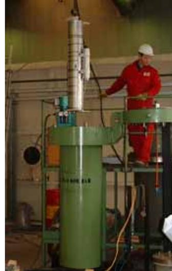
Figure 9. Installation of the instrumented riser section in the hyperbaric chamber.
