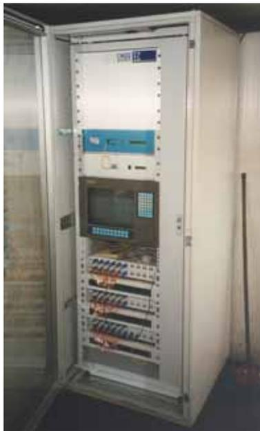
Figure 5. SOFO system for static and dynamic measurements.
