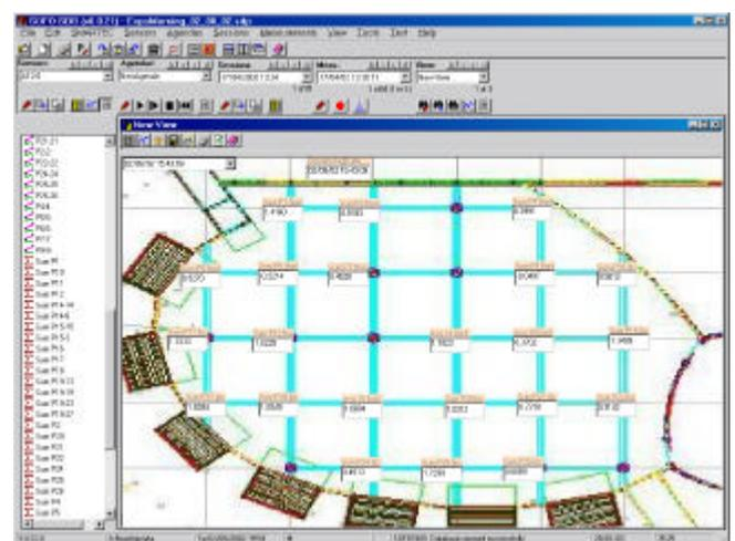
Figure 5: Piazza Pinocchio control center with load indicators
