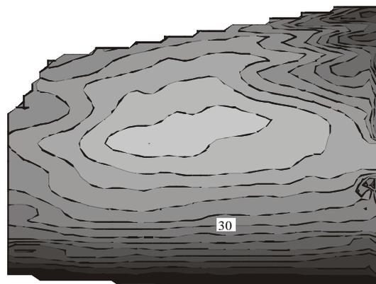
Figure 10: Temperature measurements in the Luzzone Dam 15 and 55 days after concrete pouring (courtesy of L. Thévenaz)
