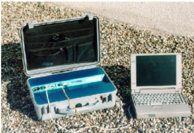
Figure 1: SOFO system reading unit
