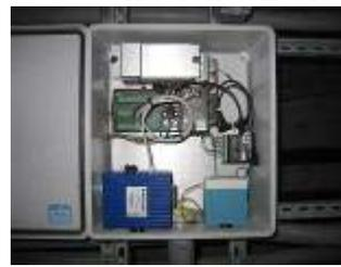
Vibrating wire and temperature sensors datalogger
