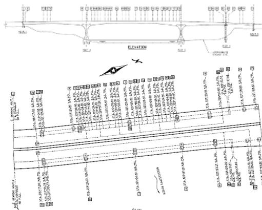
Figure 5: Location of installed instruments
