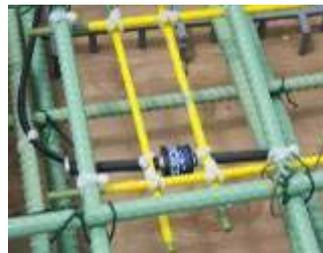
Vibrating Wire Strain Gauge
