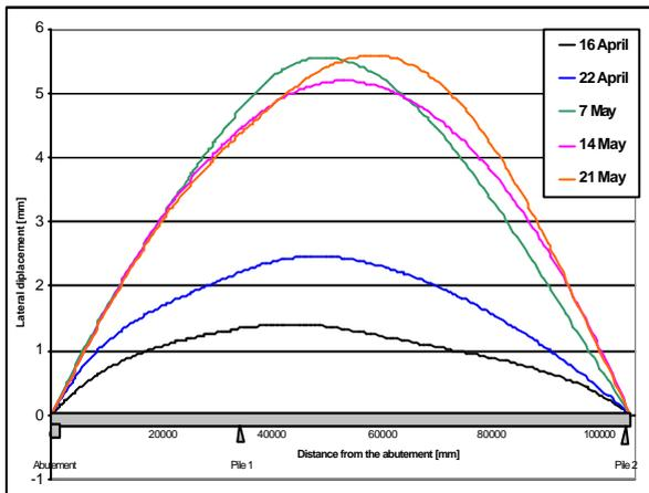
Figure 5: Evolution of horizontal displacement provoked by shrinkage of new concrete
