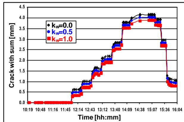
Figure 10: Evolution of crack width sum for different values of coefficient  $k_w$
