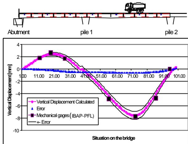
Figure 6: Vertical displacement during the load test and comparison with dial gages
