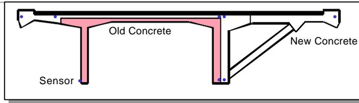
Figure 4: Position of sensors in cross-section of Versoix bridge
