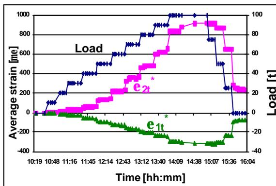
Figure 7: Evolution of load and average strains measured by sensors  $S_1$  and  $S_2$
