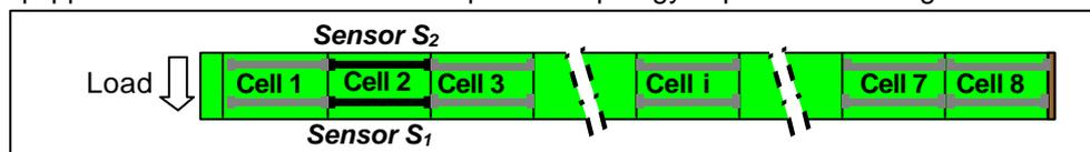
Figure 4: Schema of the pile divided in cells and position of sensors combined in parallel topology (rotated 90° in clock-wise opposite direction)
