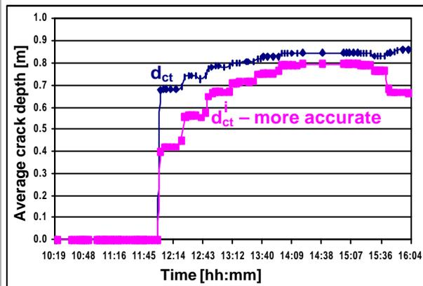
Figure 9: Evolution of average crack depth
