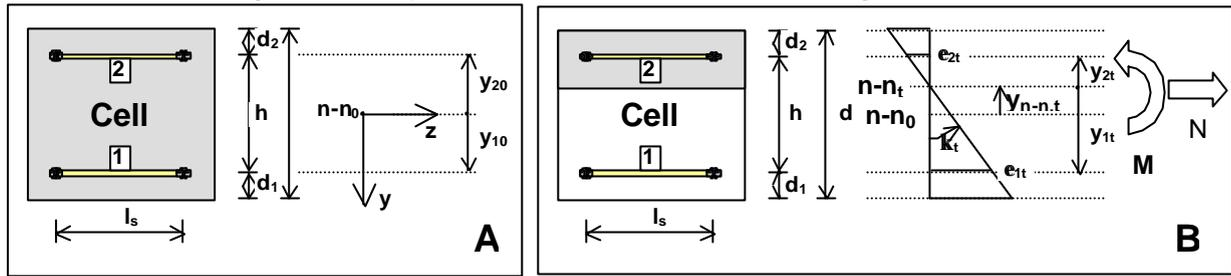
Figure 3: Parallel topology in a segment of non-cracked (A) and cracked (B) concrete beam
