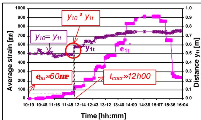
Figure 8: Determination of crack occurring time and ultimate strain of concrete
