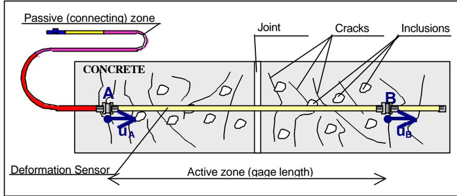
Figure 2: Schema of a long-gage sensor installed on a concrete beam with cracks, inclusions and joints
