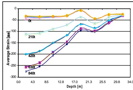
Figure 6. Average strain distribution, unloading, axial compression test.
