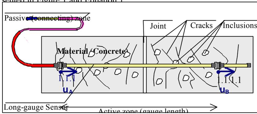
If A and B are the sensor anchoring points as shown in Figure 1, the measurement of the sensor represents a relative displacement between them. The measurement of sensor is then expressed as in Equation 1.
