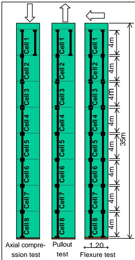
Figure 4: Topologies applied in piles monitoring and dimensions of piles
