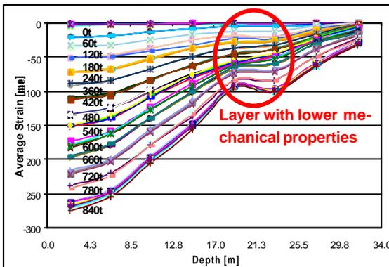
Figure 5. Average strain distribution, increase of load, axial compression test.
