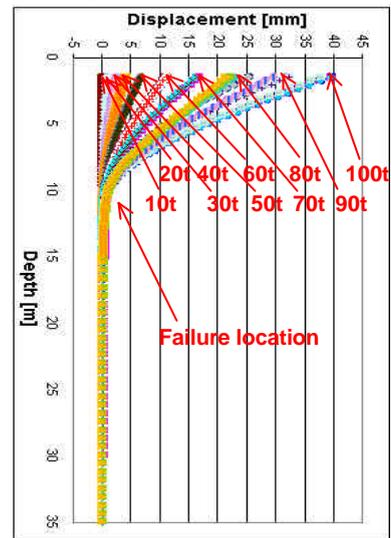
Figure 8. Deformed shapes and failure location, flexure test.
