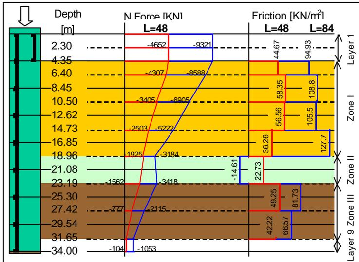
Figure 7. Distributions of normal force in the pile, friction stress and different zones of soil, axial compression test.
