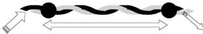
Figure 4: Microbending Sensor Functional Principle
