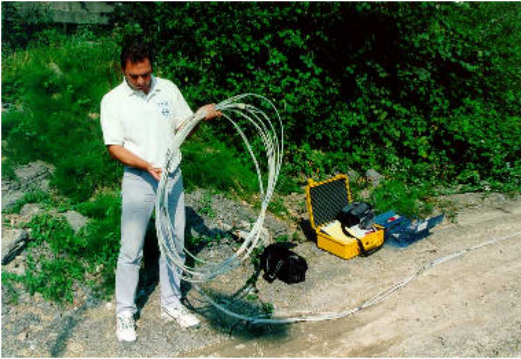
Figure 9: Bundle of SOFO Sensors Ready for Installation in a Pile for Lateral Friction Analysis
