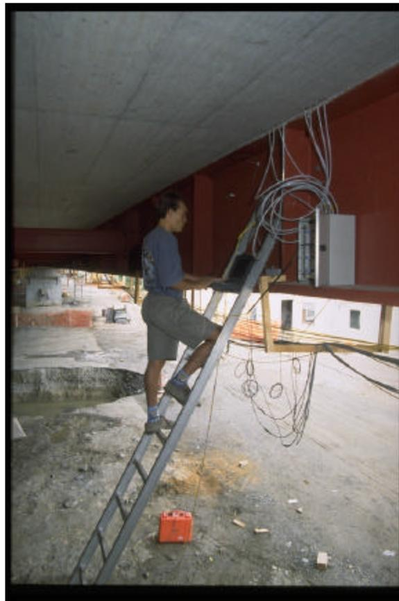
Figure 7. A typical measurement session. The operator connects the coupler to the sensor in the junction boxes and carries out the measurement with a portable PC, the reading unit remains at the bottom of the ladder.
