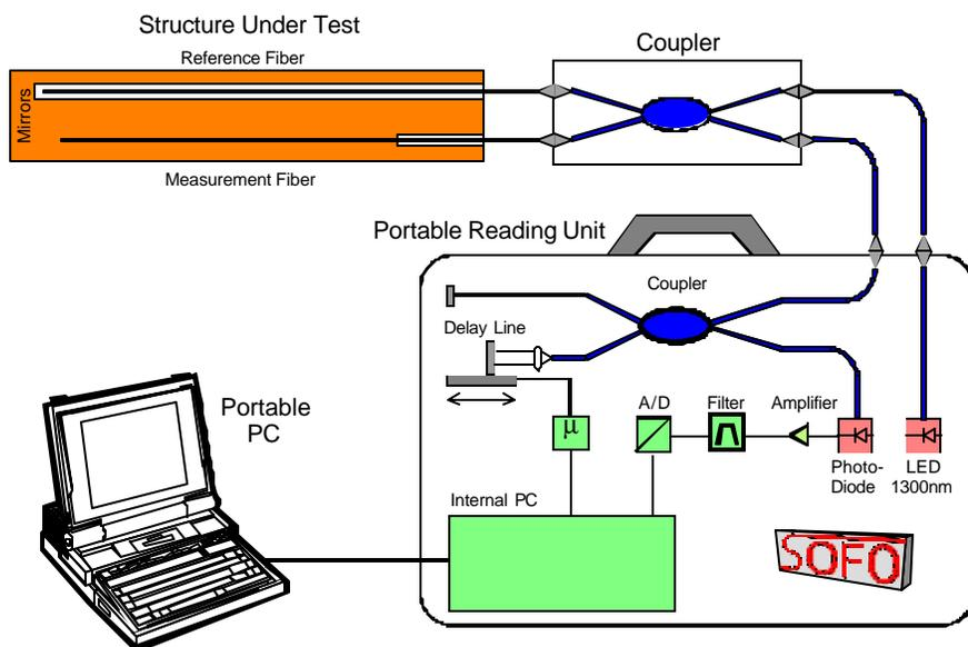
Figure 1. Optical setup of the low-coherence double interferometer. The portable reading unit is waterproof and battery powered. One measurement takes a few seconds. The temperature variation have no effect on the sensor.
