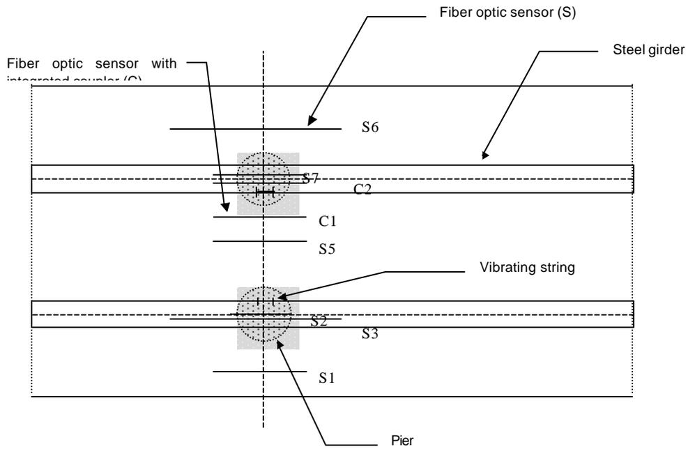
Figure 6. Section 3: Fiber optic sensor and vibrating string sensor emplacement
