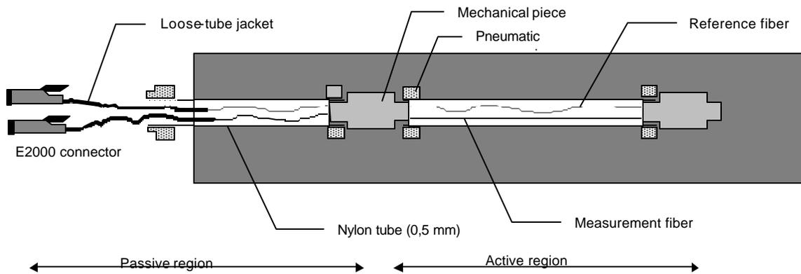
Figure 2. The SOFO sensor: schematic representation
