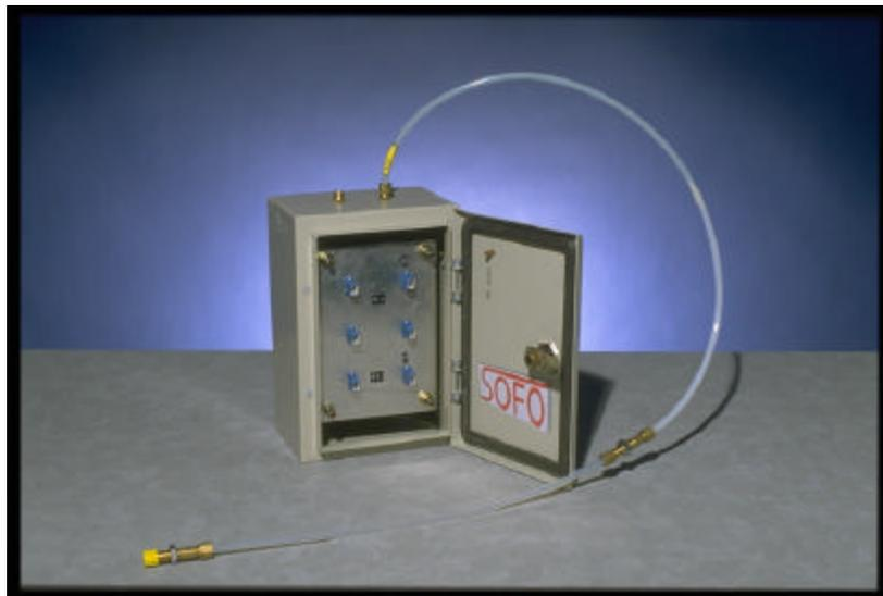
Figure 3. The SOFO sensor and its junction box
