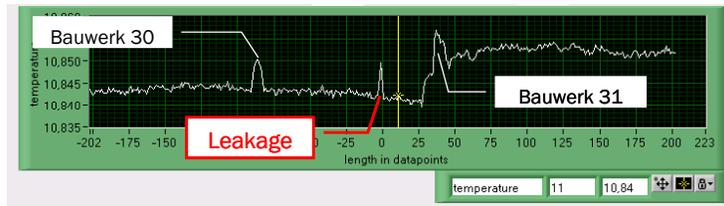
Fig. 8 Measured profiles before and after the leakage occurred at distance 17'970 meter from the pumping station, as displayed on the central PC in the control room. The vertical scale corresponds to raw Brillouin frequency shift given in GHz. The observed local temperature increase associated to the leakage was measured to be of around 8°C.
