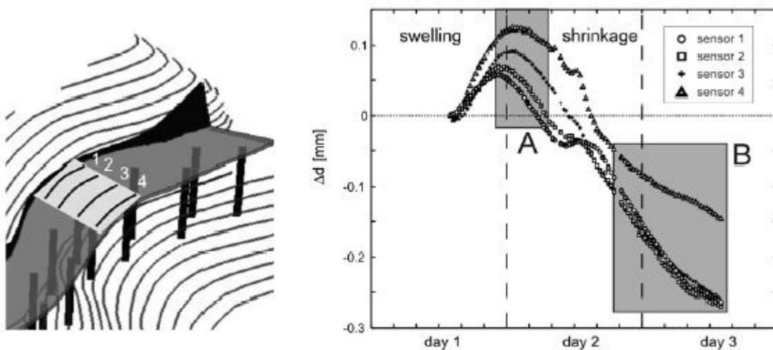
Figure 5: Measurement profile 3 (left), hardening of the concrete during the first 48 hours (right). Courtesy of Werner Lienhart and Fritz K. Brunner.
