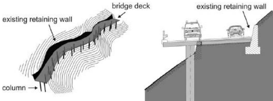
Figure 4: New bridge construction for the widening of roads in steep terrain, (Högler & Lienhart 2003)
