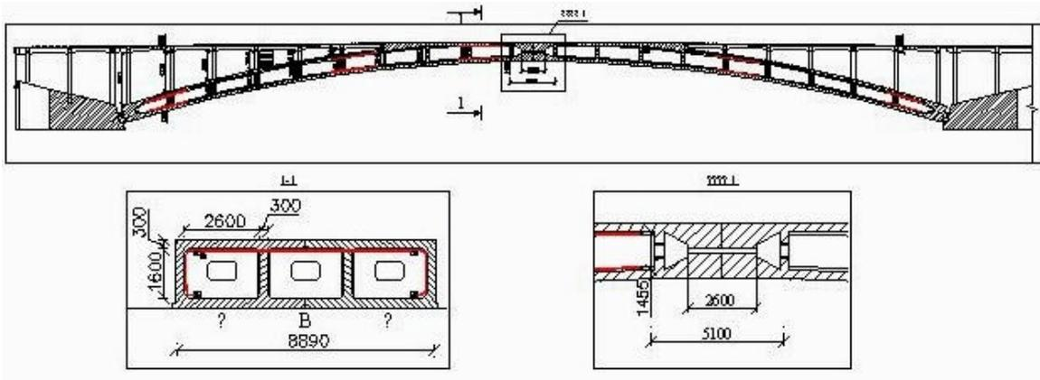
Figure 2: Bolshoi Moskvoretskiy Bridge: Longitudinal and cross sections, position of the sensors. Courtesy of Triada Holding, Moscow
