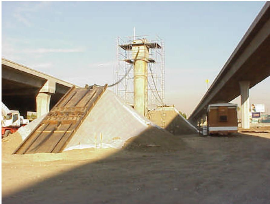
Figure 7. Bridge stack being prepared for destructive test
