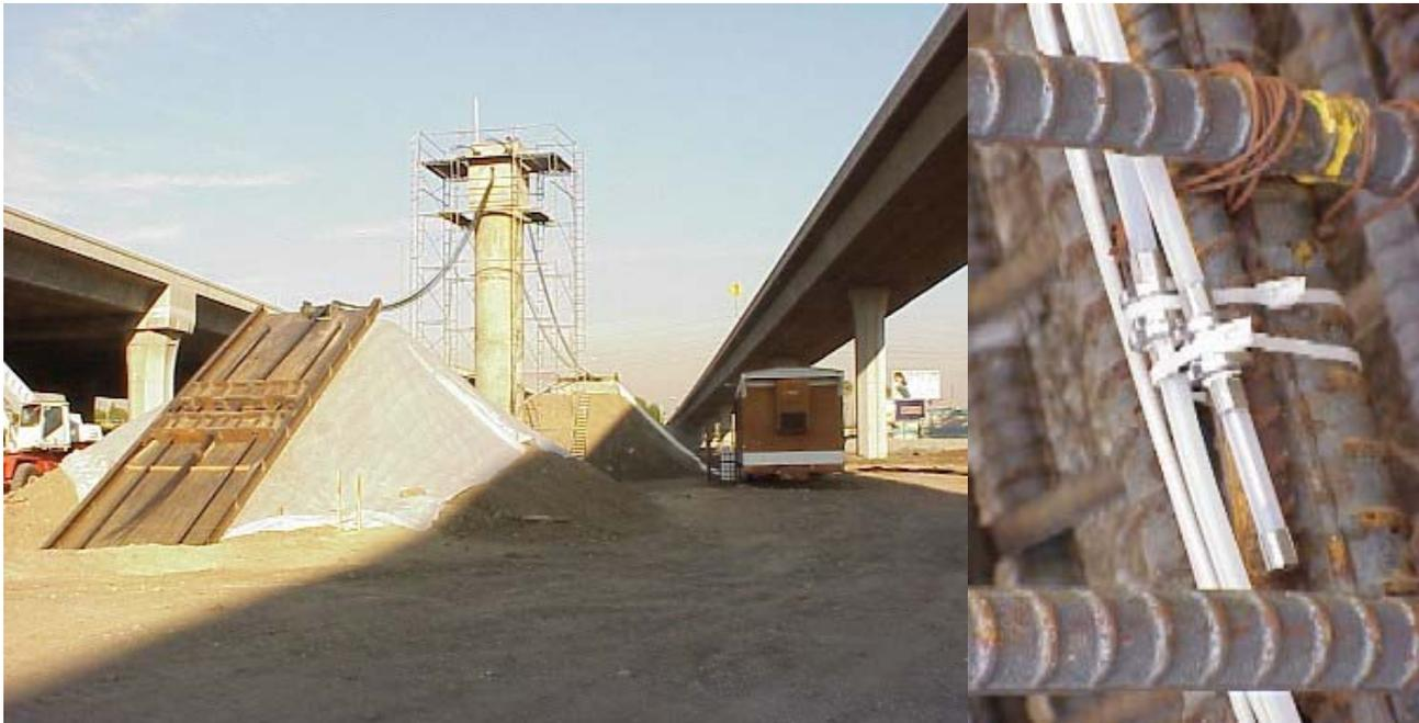
Figure 6 Bridge stack being prepared for destructive test, sensors installed on rebars.
