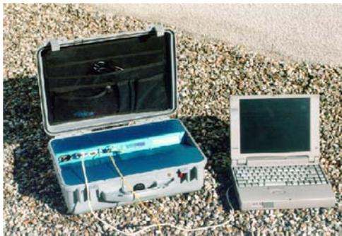
Figure 1: SOFO system reading unit
