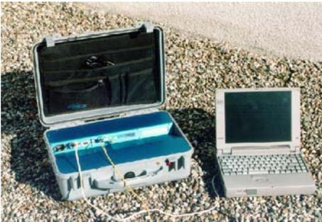
Figure 1: SOFO system reading unit
