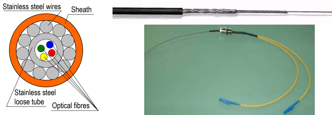
Figure 1: Extreme temperature sensing cable design and termination.
