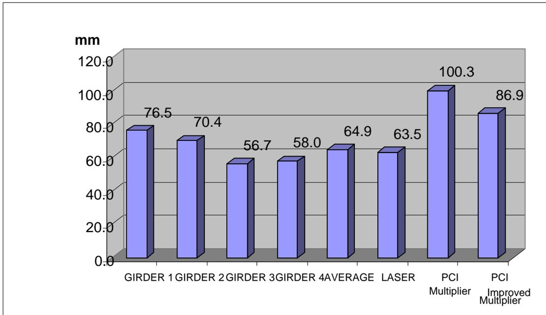
Figure 8. Girder camber at erection.
