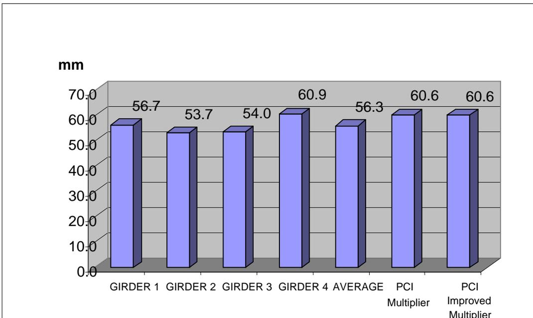
Figure 7. Girder camber right after transfer.
