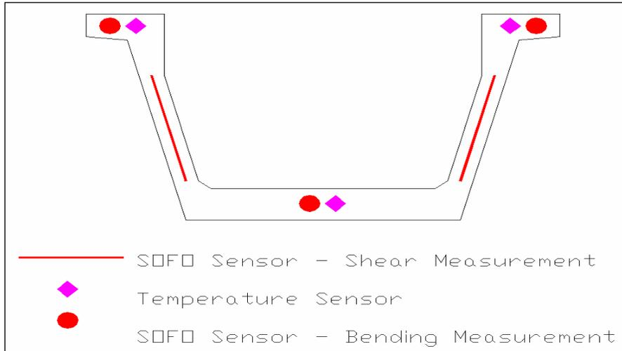
Figure 3. Girder cross-section and sensor layout.
