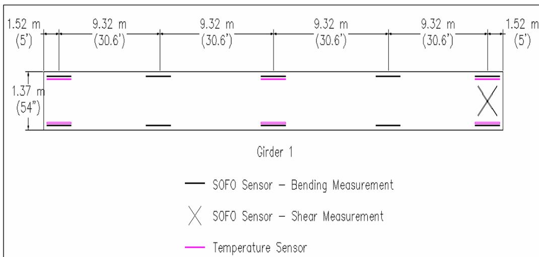
Figure 4. Elevation view of sensor layout for Girder 1.
