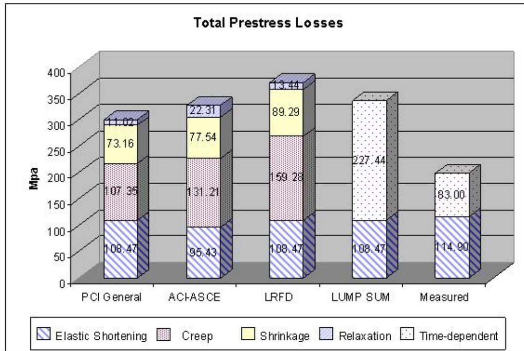
Figure 5. Comparison of the total prestress losses by all methods
