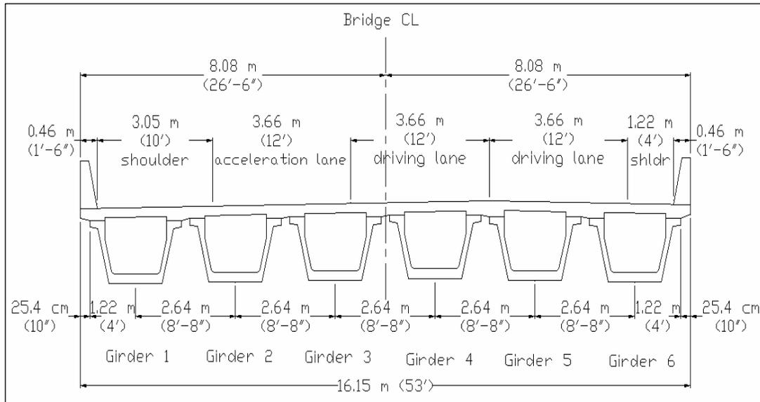
Figure 2. Deck cross-section.
