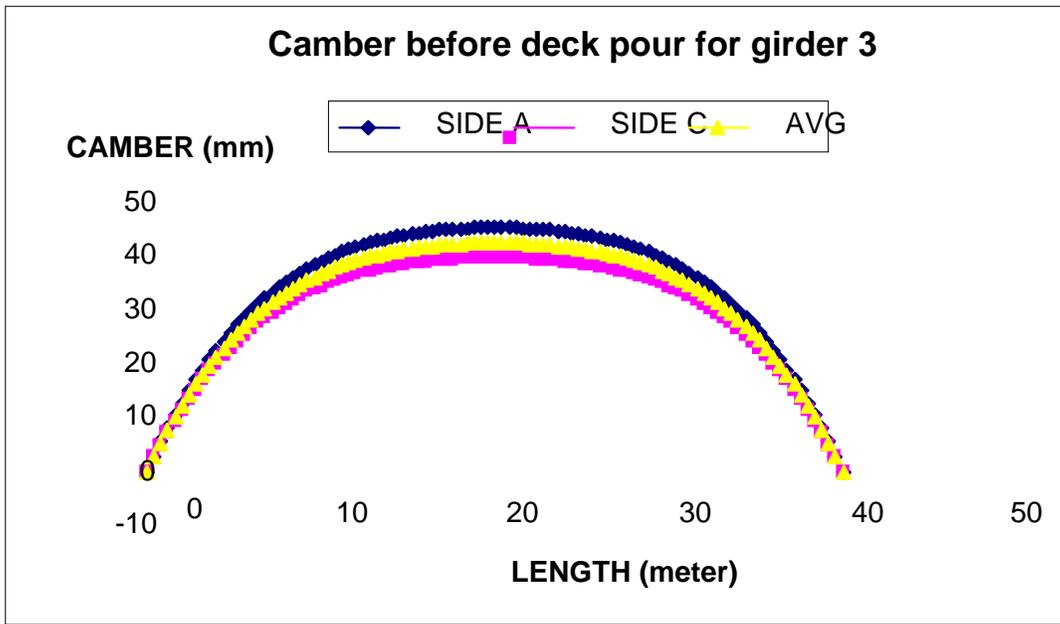
Figure 6. Typical camber plot using sensor measurements
