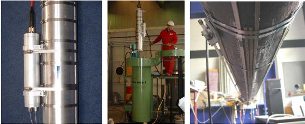
Figure 5. SOFO sensors for the monitoring of deep-water risers. SMARTprofile sensors and underwater interconnection box. Testing in hyperbaric chamber and full scale bending test.
