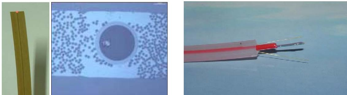
Figure 1. SMARTape for distributed strain sensing and SMARTprofile for distributed strain and temperature sensing
