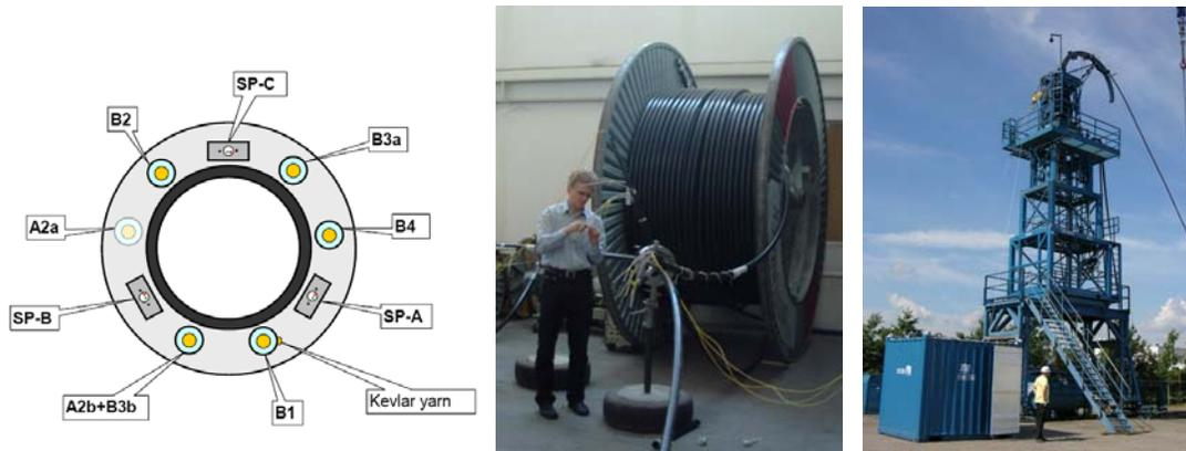
Figure 3. Cross section of the PDT-Coil Liner, including SMARTprofile sensors for strain and temperature (SP) and electrical conductors (A and B). Laboratory testing with current injection and field testing using steel coiled tubing equipment.
