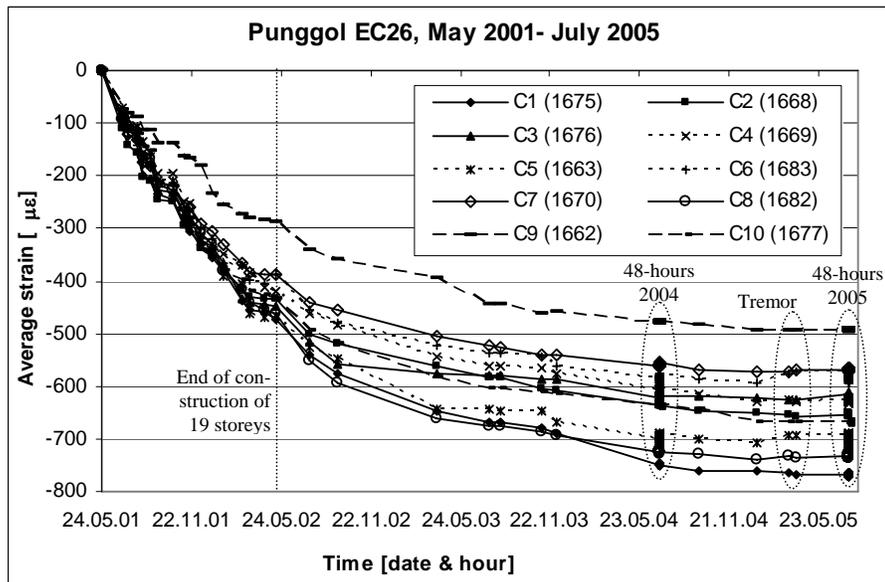
Figure 4. Evolution of total average strain in columns monitored by SOFO system
