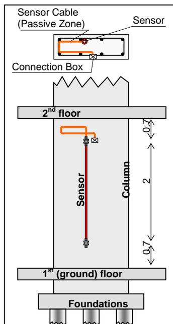
Figure 2. Sensor position in column
