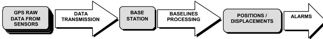
sensors and stored in local memory. The baseline processor is responsible for post-processing the raw measurement data. The data is processed in batch, and the result consists of the positions of the various moving sensors relative to the reference sensors. The base station may optionally be equipped with an uninterruptible power supply (UPS) to bridge power brownouts or blackouts. A local, standard precision GPS receiver serves to download satellite visibility data (the almanach).
