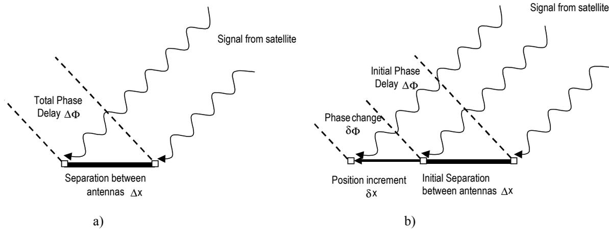
Figure 1: Separation between two GPS antennas is measured from the total phase delay between the received carrier signals.
