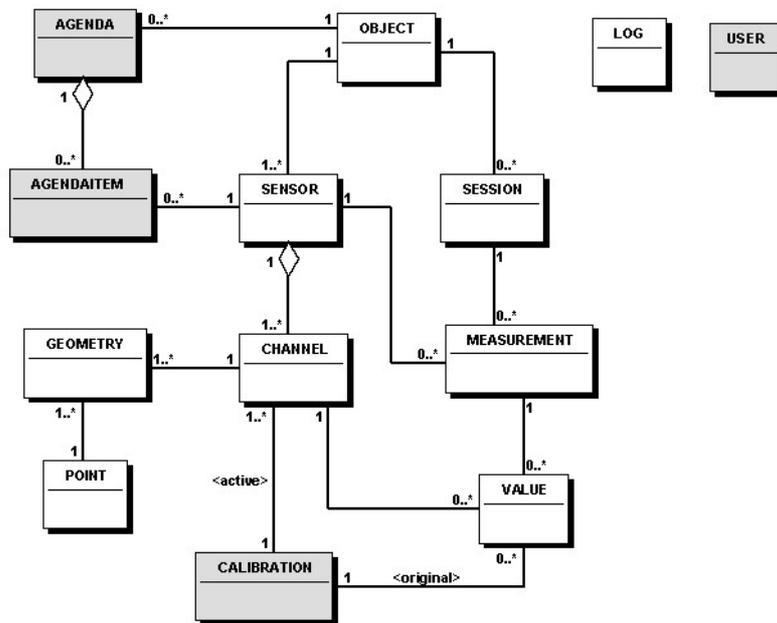
Figure 5: Entity Relationship Model using the UML notation
