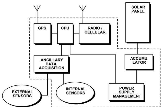
Figure 3: Sensor unit block diagram.
