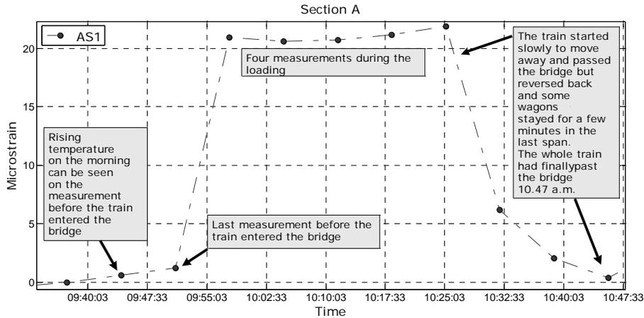
Figure 3. Strains in a 4 meter long sensor located in the outer edge of the eastern cantilever in longitudinal direction.
