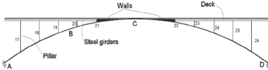
Figure 7. Side view and parts of the bridge that were rebuilt under the retrofitting
