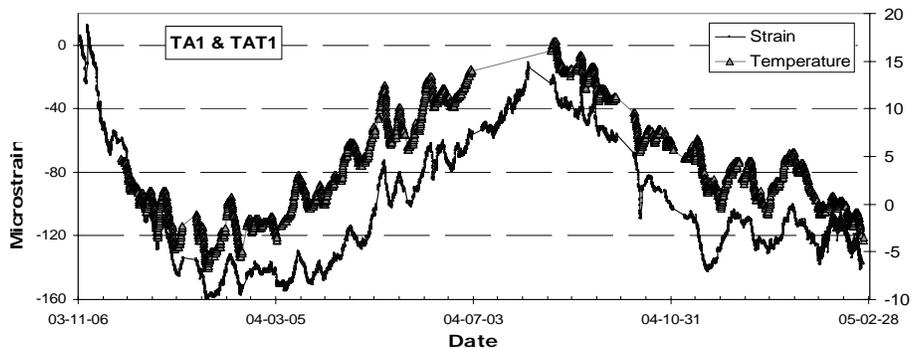
Figure 8. Strain and temperature profiles during the retrofitting period of about 16 months.
