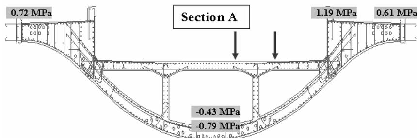
Figure 4. Maximum tensile (+) and compressive (-) stresses at section A.
