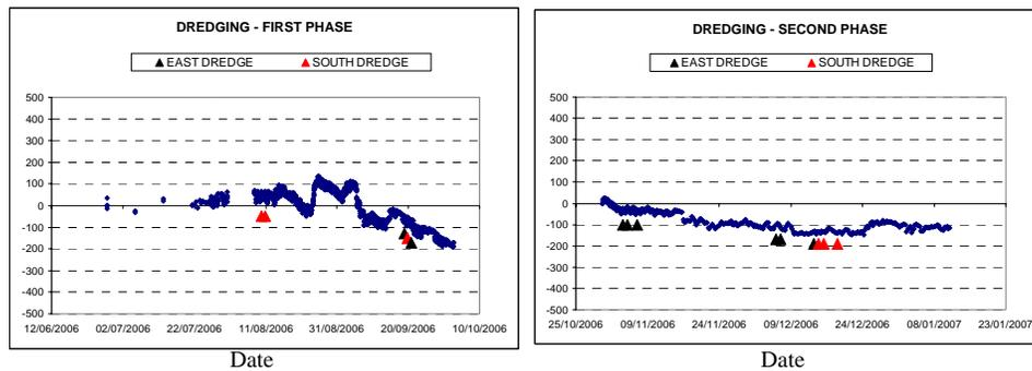
Figure 6. Strain variation (in microstrain) of a tendon in the corner during the two phases of dredging.
