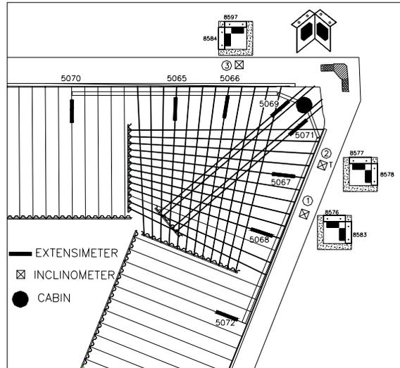
Figure 5. Fibre Bragg grating on the tendons and location of inclinometers in the south-east corner of the pier.
