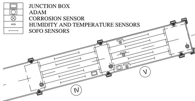
Figure 7. Location of sensors in typical pier spans.
