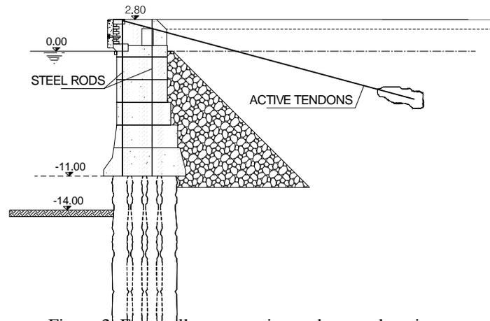
Figure 2. East wall cross-section and sensor location.
