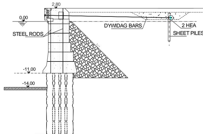
Figure 4. Wall cross-section and strengthening works.
