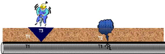
**Fig.3.** Detection of a gas leak through a cable placed above the pipeline. This arrangement can also be used to detect a third-party intrusion.
