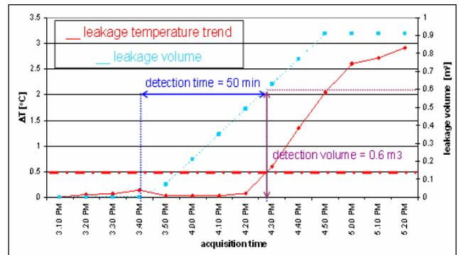
Fig.7. temperature and leaked volume evolution at leak location 3.
