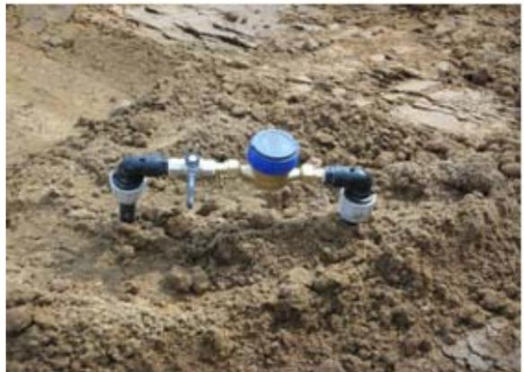
**Fig.4.** Leakage detection simulation arrangement. Warm water is injected in the ground at different positions with respect to the sensing cable position. Several taps, with volume meters are used to generate controlled leaks.
