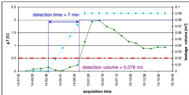
**Fig.9.** Temperature and leaked volume evolution at leak location D5, 2<sup>nd</sup> test with  $\Delta T=3^{\circ}\text{C}$ .
