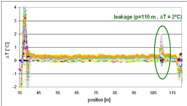
**Fig.8.** Relative temperature data for the leakage test. The temperature peaks from the leakage is clearly visible.
