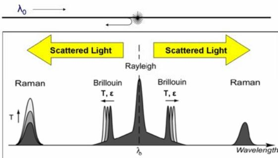
Fig.1. Light scattering in optical fiber
