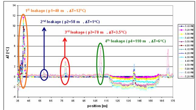
Fig.6. Relative temperature data for the leakage test. The temperature peaks from the four leakages are clearly visible.
