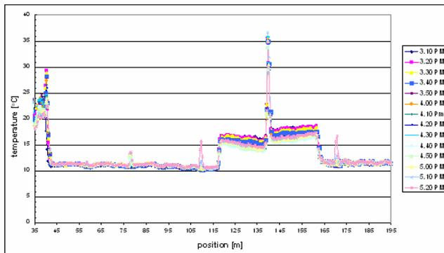
Fig.5. Raw temperature data for the leakage test.
