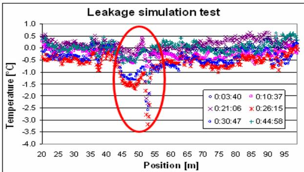
**Fig.11.** Temperature drop due to gas pressure release indicates the presence of a leakage.
