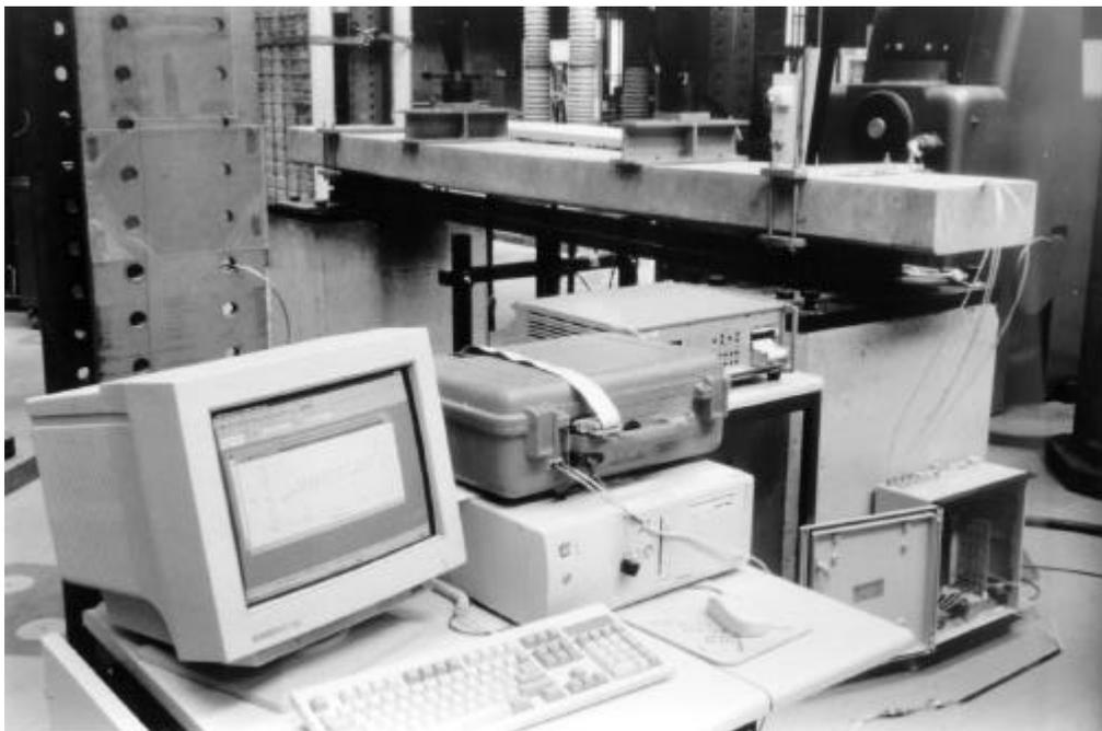
Figure 1: Concrete beam subject to cyclic four-point-bending. The SOFO system is visible in the foreground.
