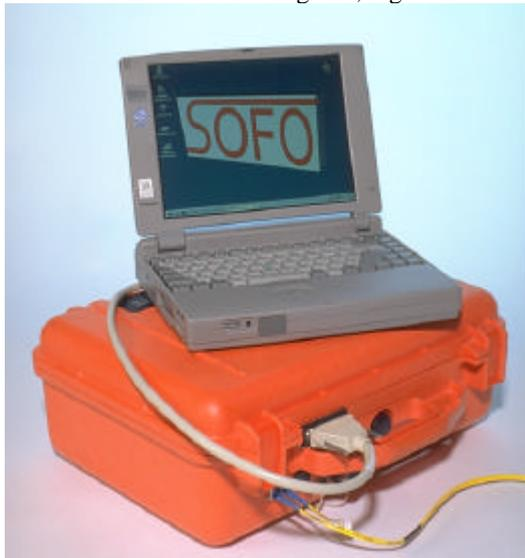
Figure 3: SOFO reading unit with external control PC.
