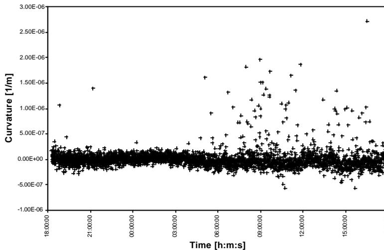
**Figure 13: Curvature data after removing the bridge's temperature drift.**
