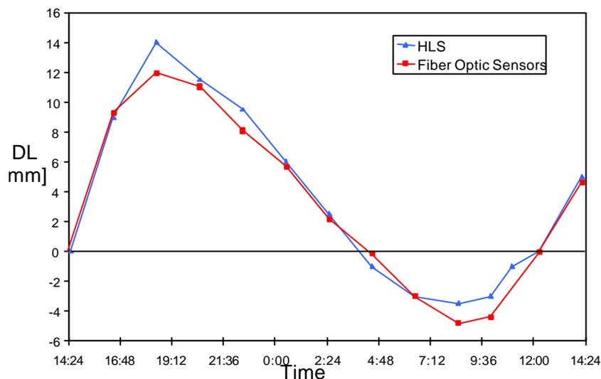
**Figure 11: Vertical displacement of the Lutrive Bridge calculated by double-integration of the curvature measurements.**
