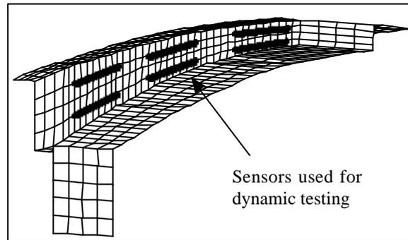
**Figure 10: SOFO sensors placement**
