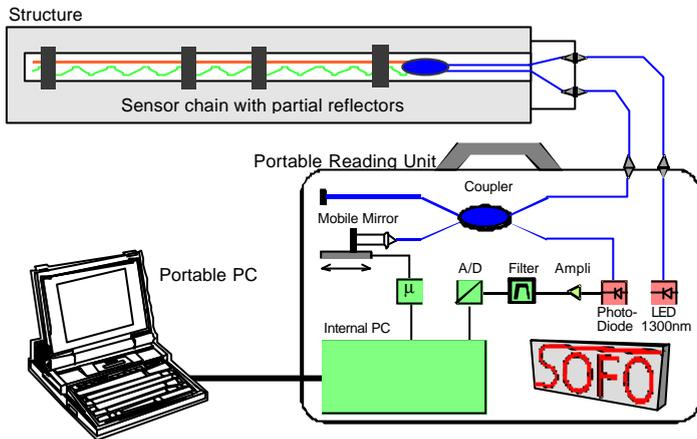
Figure 1: Setup of the SOFO system.
