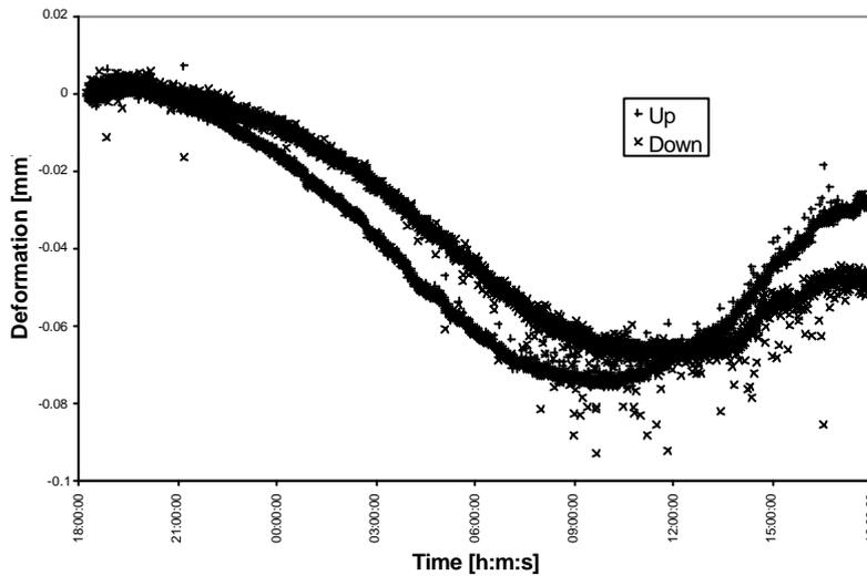
**Figure 12: Deformation data obtained on two parallel sensors placed at quarter-span in the Lutrive bridge.**
