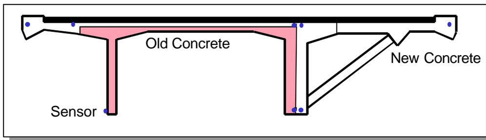
**Figure 4: The Versoix Bridge cross-section and placement of the sensors**
