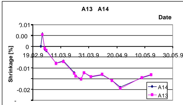
Figure 11: Differential shrinkage between the old and new concrete
