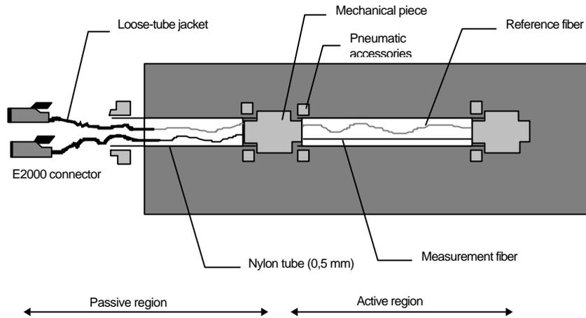
**Figure 2: Setup of the SOFO sensors**
