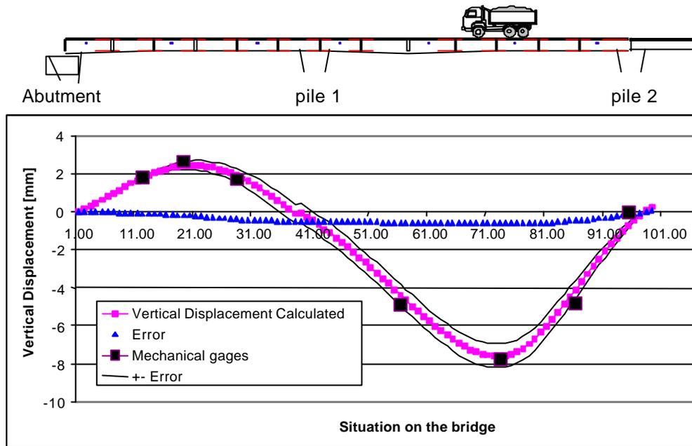
Figure 13: Vertical displacement, load case A
