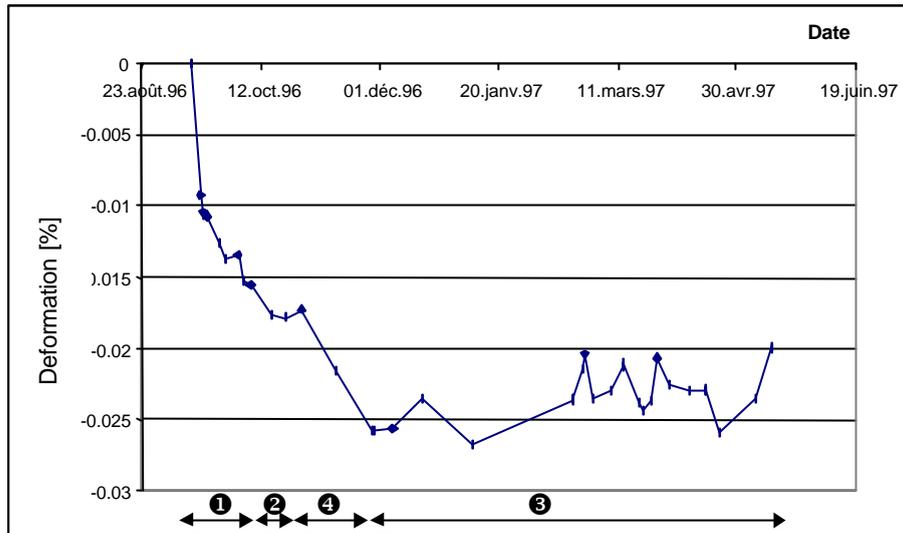
Figure 9: Typical deformation measurement over 8 months
