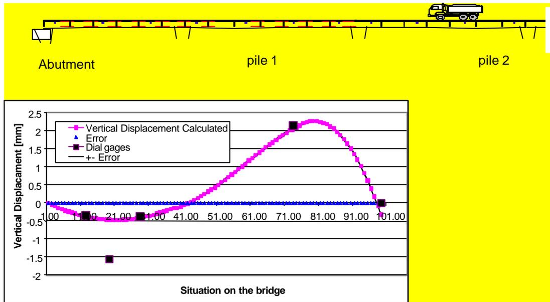
Figure 14: Vertical displacement, load case B
