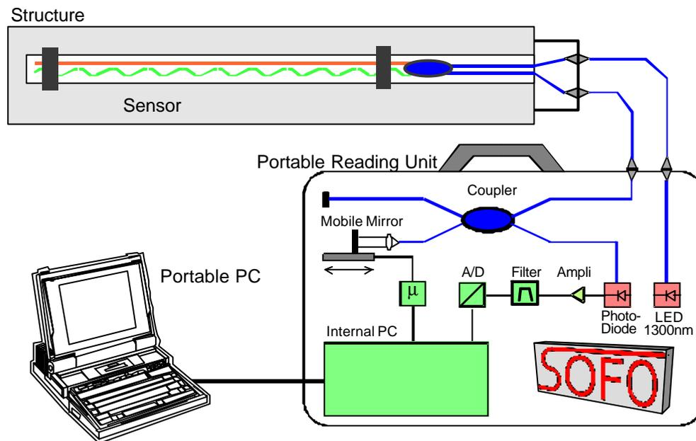
Figure 1: Setup of the SOFO system
