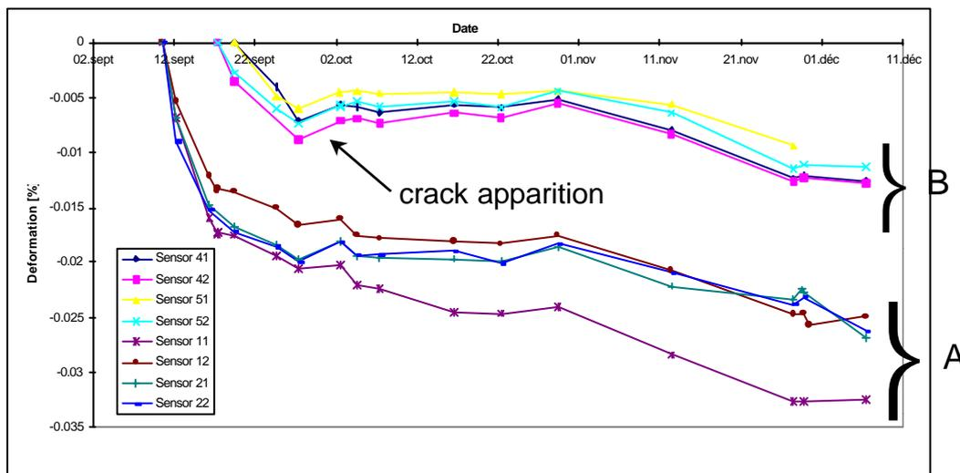
Figure 10: Comparison between cracked and un-cracked sections
