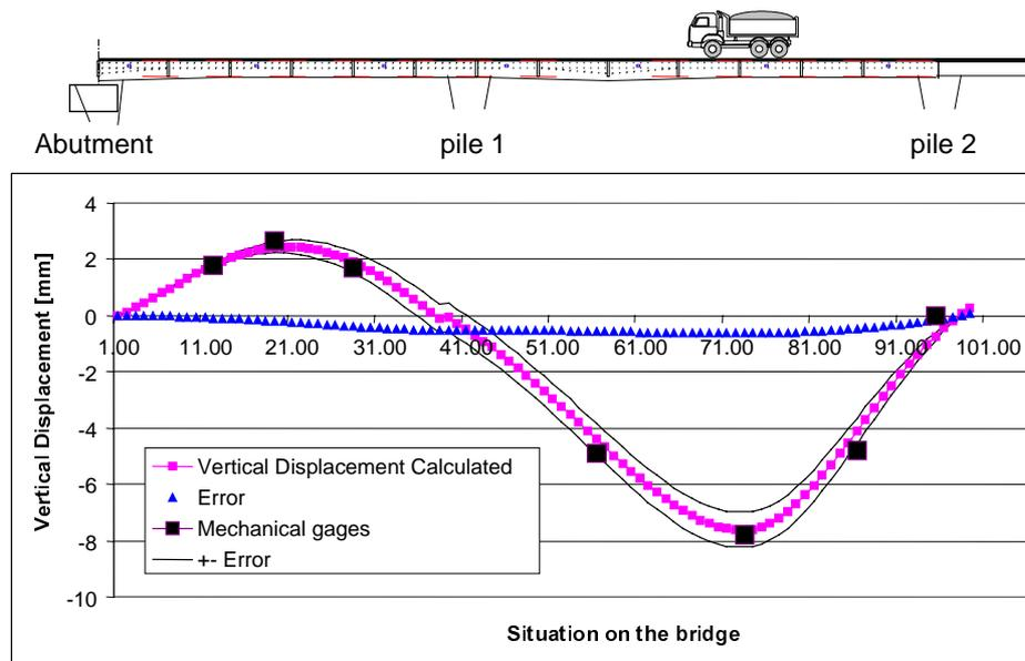
Figure 4: Vertical displacement, load case A
