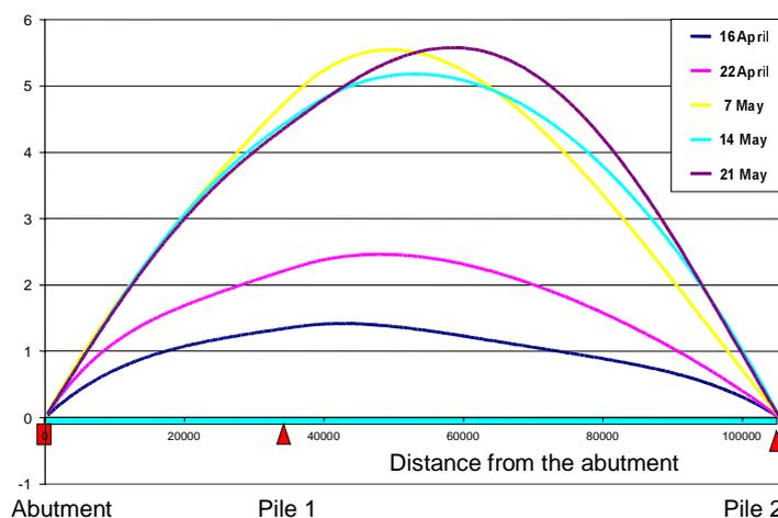
*Figure 3: Horizontal displacement of the bridge*
