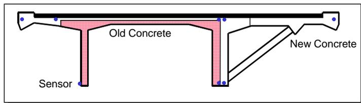
Figure 1: The Versoix Bridge cross-section and placement of the sensors
