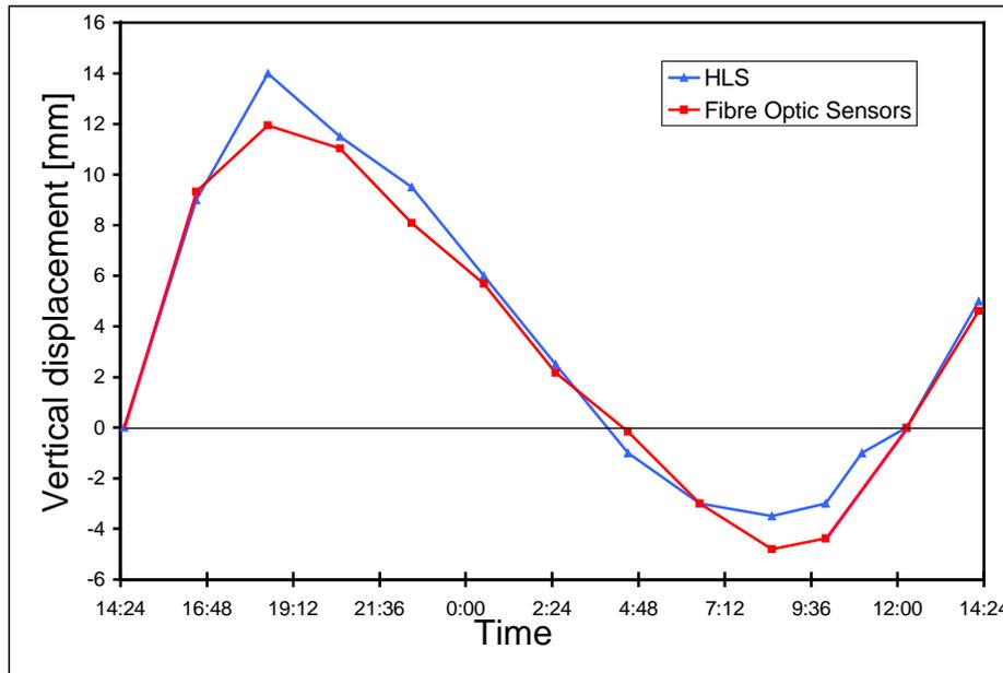
Figure 6: Vertical displacement at quarter span under thermal loading
