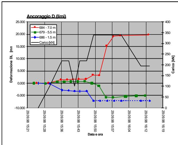
Figure 12 Load test on anchor D
