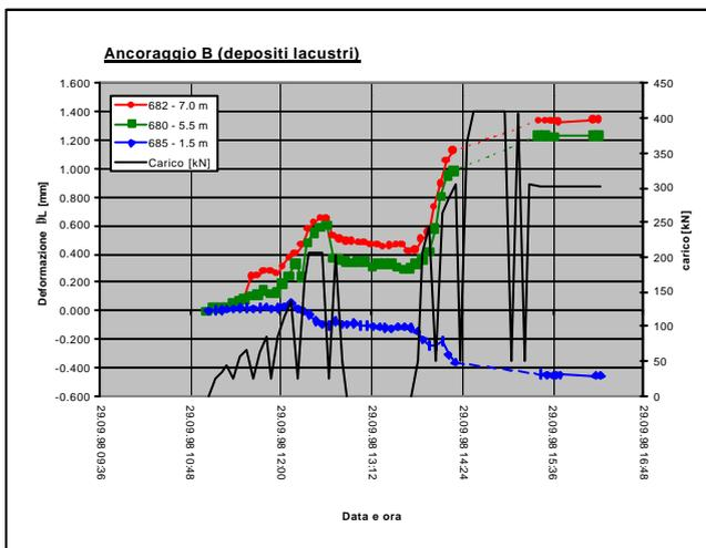
**Figure 10 Load test on anchor B**
