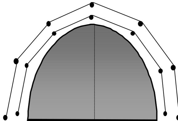
**Figure 6 Installation of sensors for curvature measurement and convergence analysis.**
