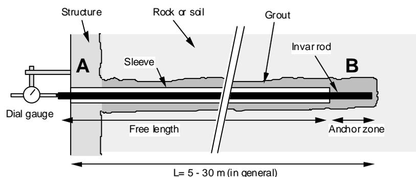
**Figure 4 Schematic representation of a conventional extensometer; the measurement will give the relative displacement between points A and B**
