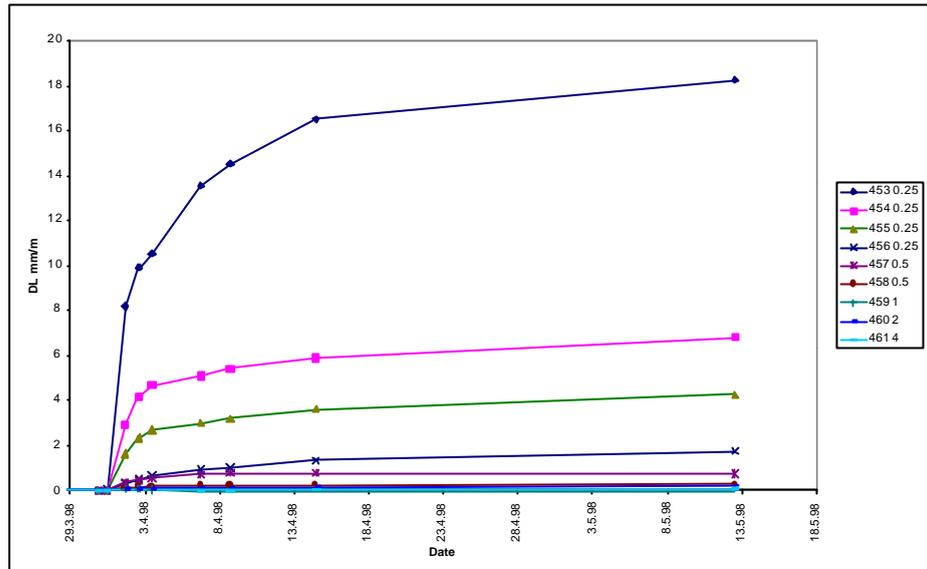
**Figure 8 Strain measurement in the Mt. Terri Tunnel.
