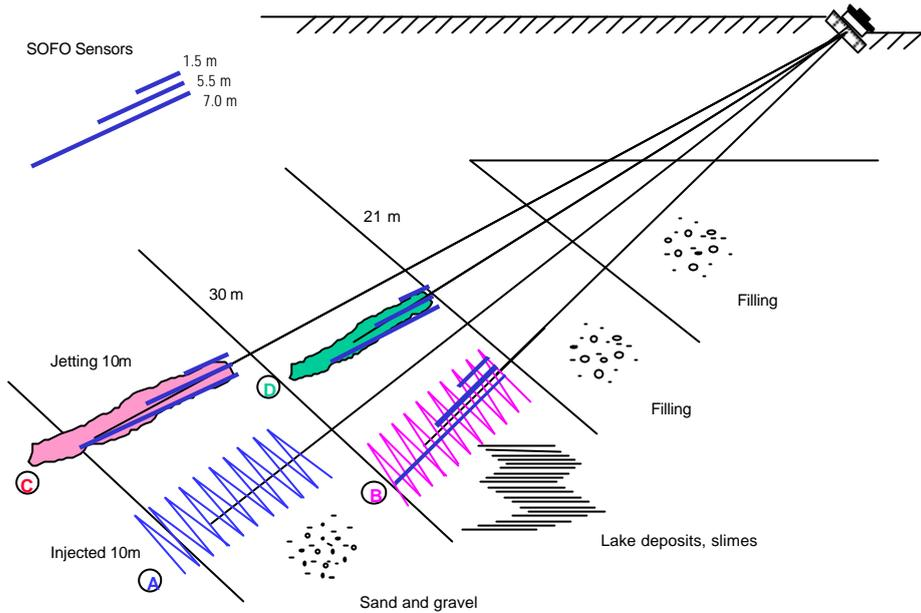
**Figure 9 Schematic representation of the 4 test anchors (B, C e D have been instrumented with SOFO sensors)**
