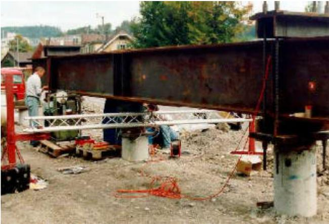
Figure 14 Pile loading setup
