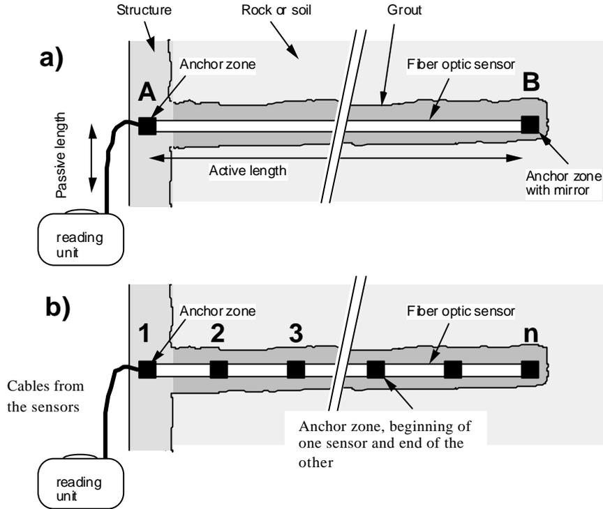
**Figure 5 Schematic representation of our fiber optic extensometer;**
