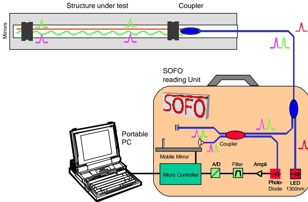
**Figure 1 Setup of the SOFO system**
