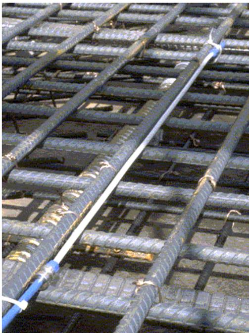
**Figure 2 SOFO Sensors installed on a rebar**
