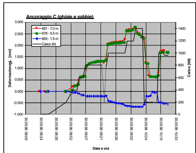
**Figure 11 Load test on anchor C**
