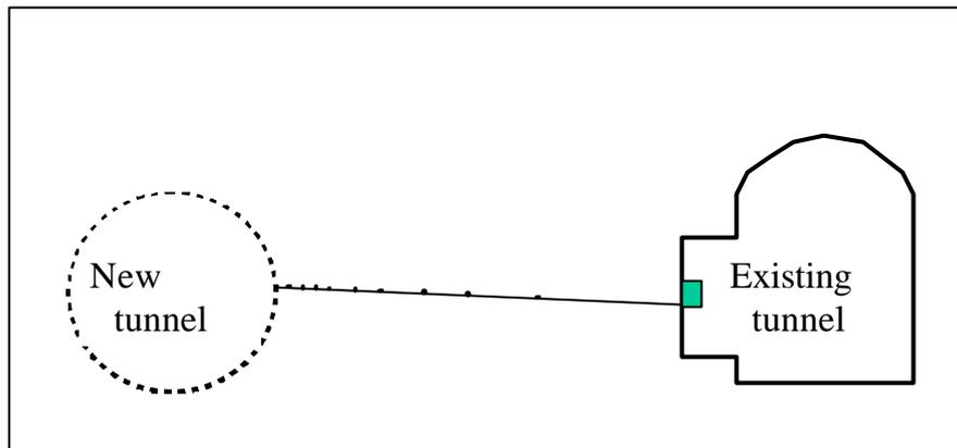
Figure 7 Sensor installation in the Mt. Terri tunnel.
