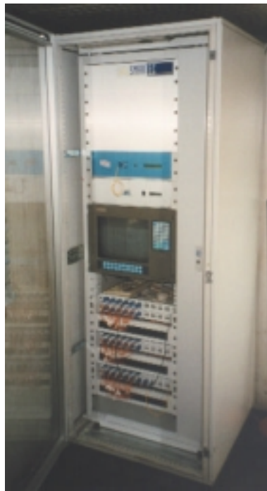
Figure 5 SOFO reading unit , optical switch, control PC and cable connections
