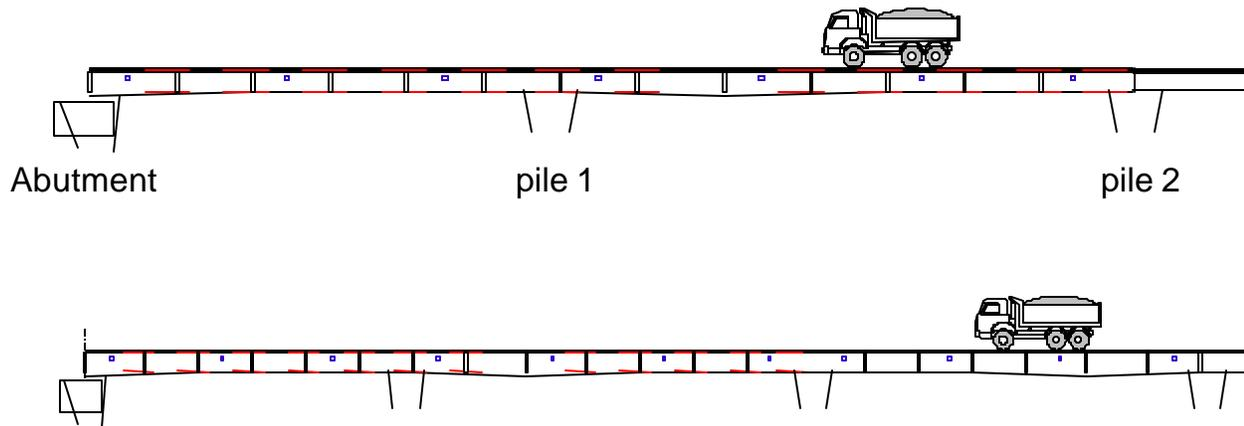
*Figure 12 : Load test A and B*
