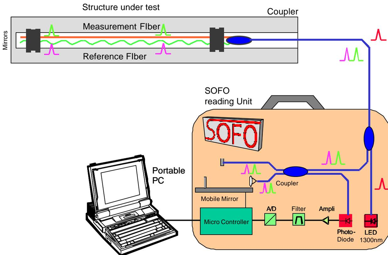
*Figure 3: Optical setup of the SOFO system. The portable reading unit is waterproof and battery powered. The Sensor is made up of a reference fiber which is free and a measurement fiber which is attached to the structure.*
