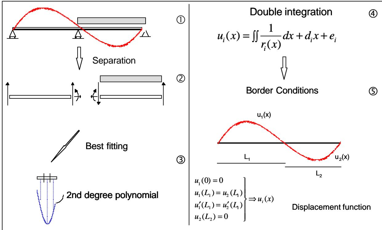
Figure 4: General description of the algorithm. Vertical shape is retrieved by a double integration of the measured curvature function.
