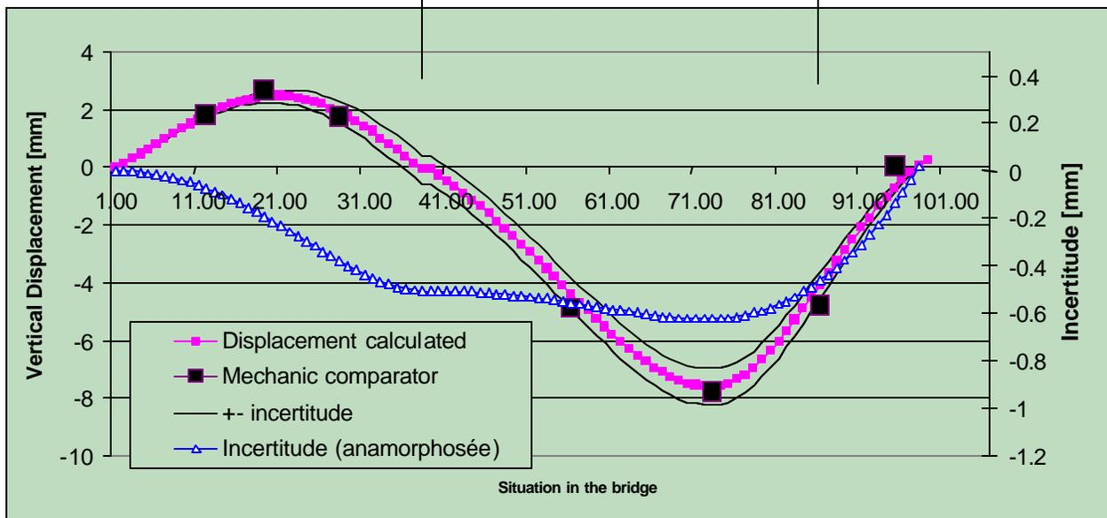
Figure 14 : Comparison of the vertical displacement calculated and the incertitude for the load case A.
