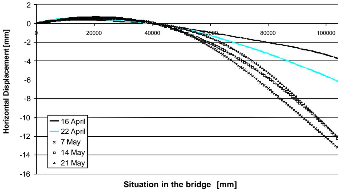
Figure 11 : Horizontal displacement evolution. The free point is at pile2
