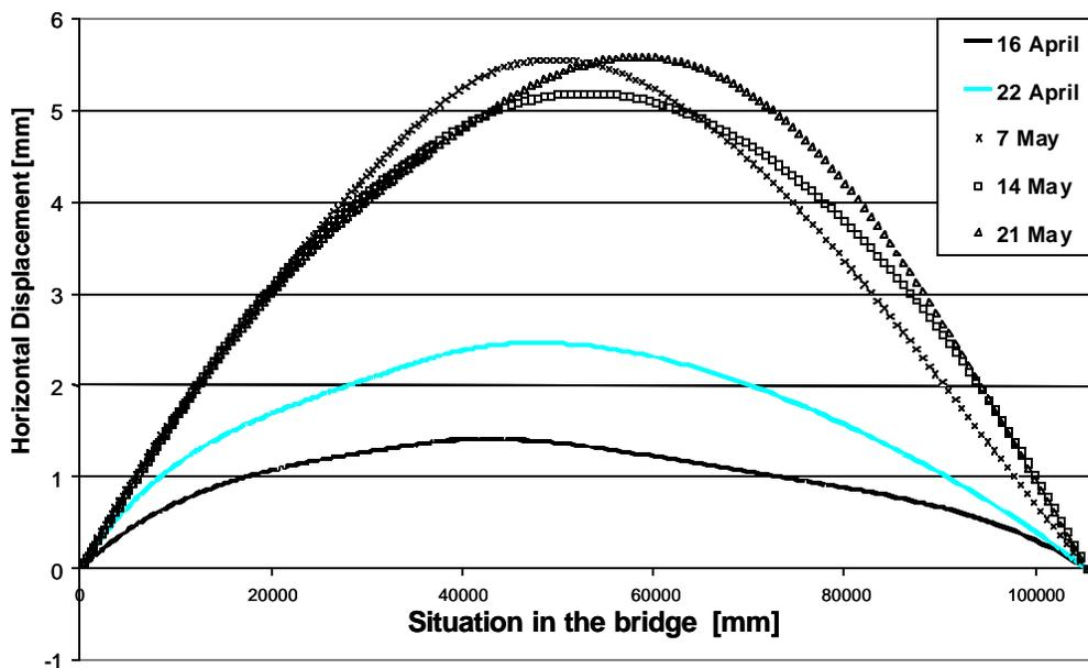
Figure 10 : Horizontal displacement evolution. The free point is at pile 1
