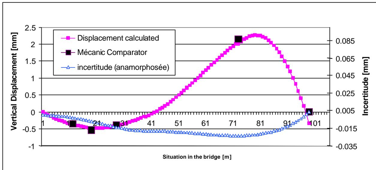
Figure15 : Comparison between the algorithm and the mechanical comparator for the load case B
