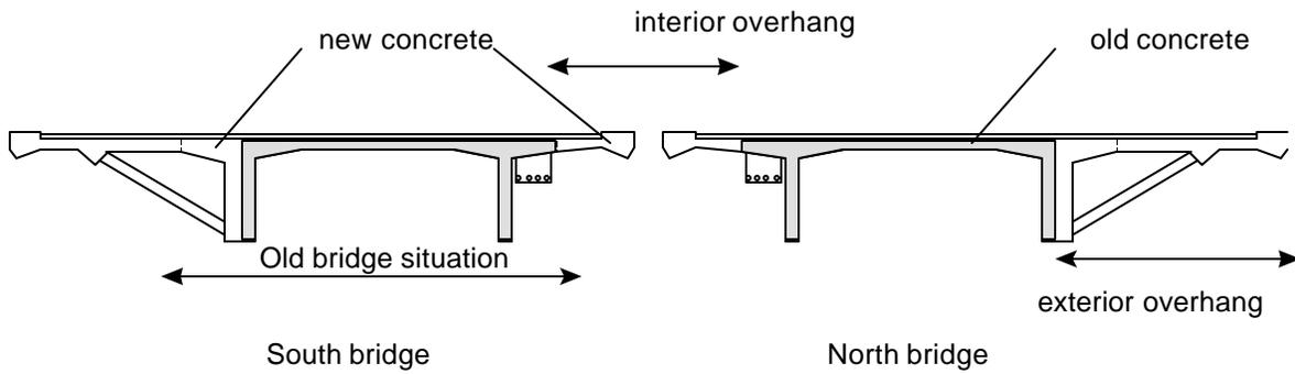
Figure 5: The north and south Versoix bridge: widening principle
