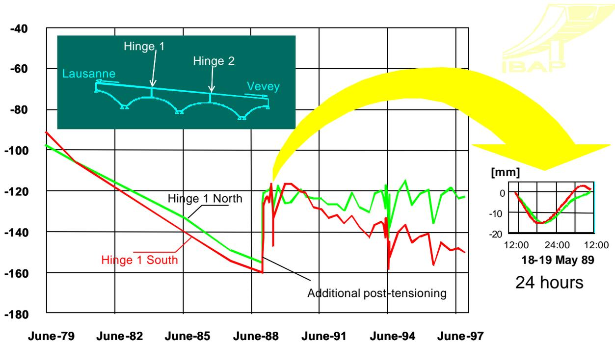
Figure 2: Vertical displacement of the Lutrive Bridge since July 79. The Daily temperature effect in the bridge vertical deflection is showed at right.
