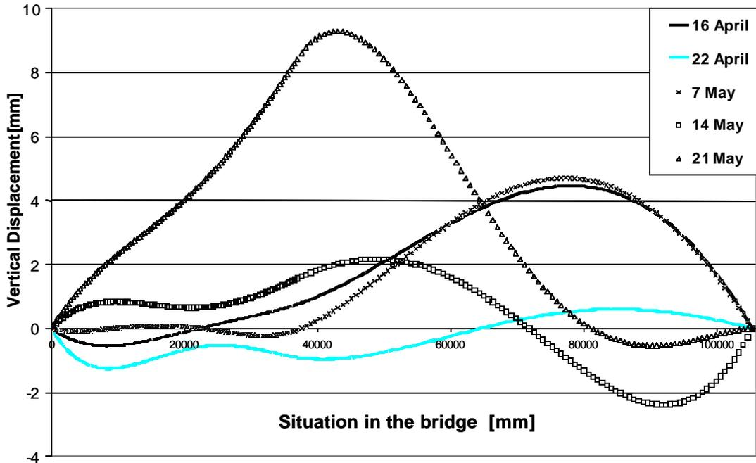
Figure 9 : Evolution of the vertical displacement of the two spans
