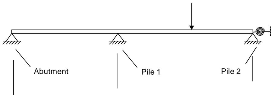
Figure 13 : Static modelisation of the 2 spans analysed on the load case A
