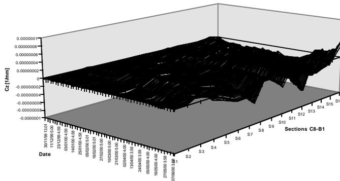
Figure 7: Time-curvature-space plot for the entire wall.
