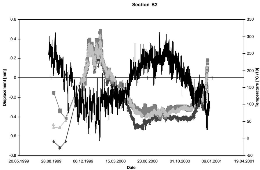
Figure 3: Time-strain-temperature plot for a section out-of-phase with thermal variations.
