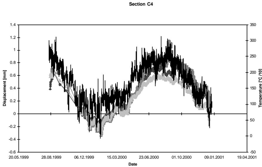
Figure 2: Time-strain-temperature plot for a section in-phase with thermal variations.
