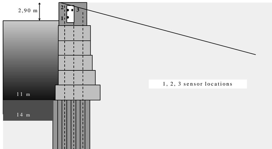
Figure 1: Quay wall cross-section; strengthening works and sensor locations.
