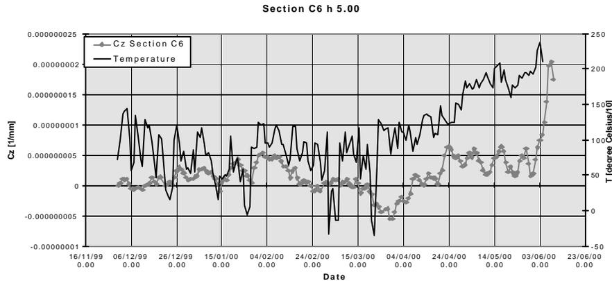
Figure 6: Time-curvature-temperature plot for the same hour.
