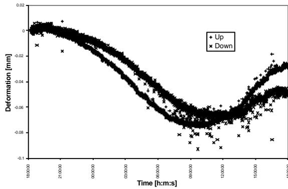
Figure 3 Deformation data obtained on two parallel sensors placed at quarter-span in the Lutrive bridge.
