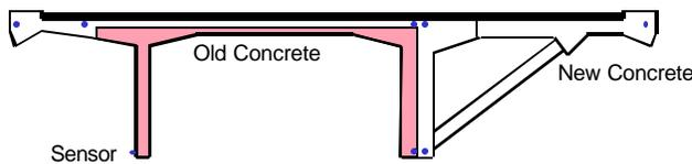
Figure 7 Sensor placement in the bridge cross-section. The red part represents the old concrete. Notice the sensor pairs in the right beam.
