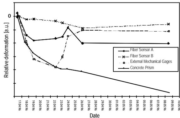
Figure 6 Measurements on the SOFO<sup>®</sup> sensors, on the mechanical extensometer and on the concrete prisms
