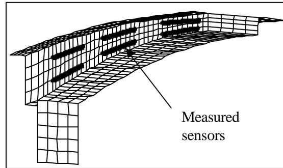
Figure 2 Sensor placement for monitoring the Lutrive bridge. The setup is repeated on the other side of the bridge
