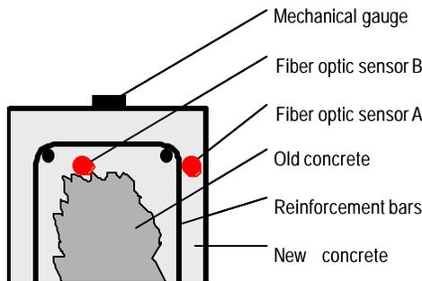
Figure 5 Cross-section of the refurbished beam and placement of the sensors
