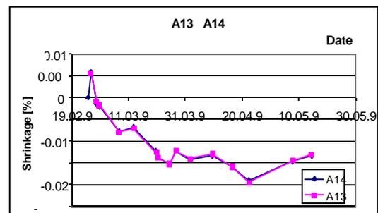
Figure 8 Differential shrinkage between old and new concrete. No relative movement is visible indicating that the bridge is acting monolithically
