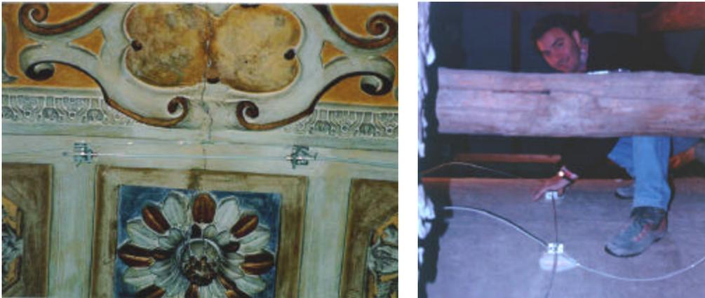
Figure 4: SOFO sensor installed underneath and above the Gandria Church vault
