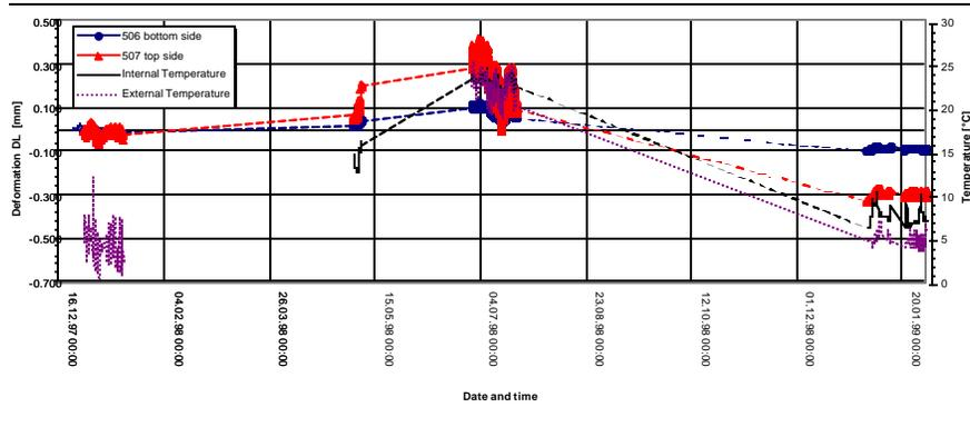
Figure 6: Long-term monitoring of the Vaults deformations, internal and external temperatures
