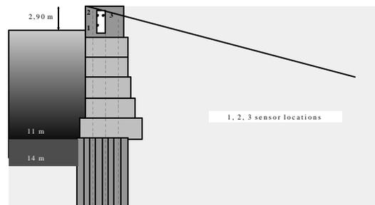
Figure 8: Quay wall cross-section, strengthening works and sensor locations.
