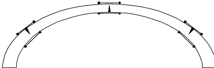
Figure 3: Location of the main cracks and SOFO sensor layout
