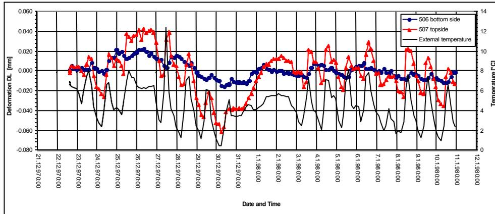
Figure 5: Measurement of two sensors above and below the vault and to the air temperature during three weeks.
