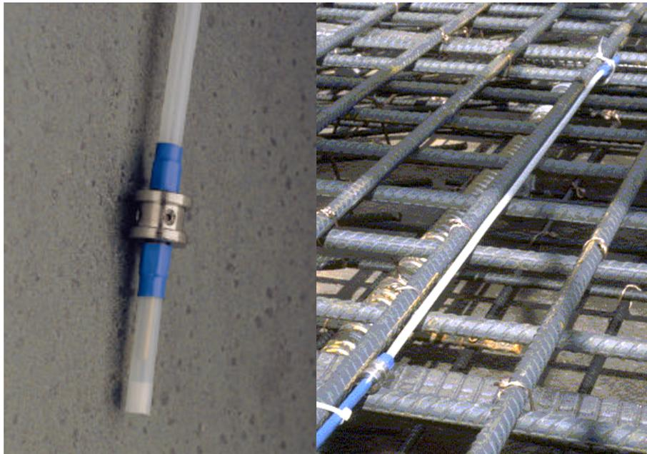
Figure 2: SOFO fiber optic deformation sensor
