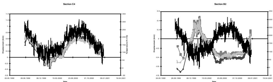
Figure 9: Time-strain-temperature plot for a section in-phase and out-of-phase with thermal variations.
