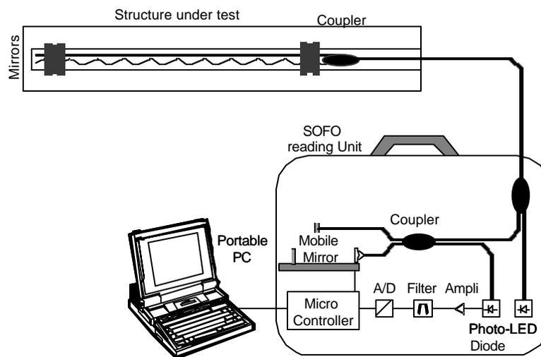
Figure 1: Setup of the SOFO system
