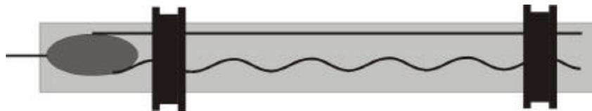
**Figure 7. SOFO Fiber optic sensor**
