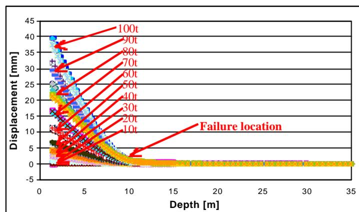
Figure 7. Deformed shapes of the pile and identification of failure location
