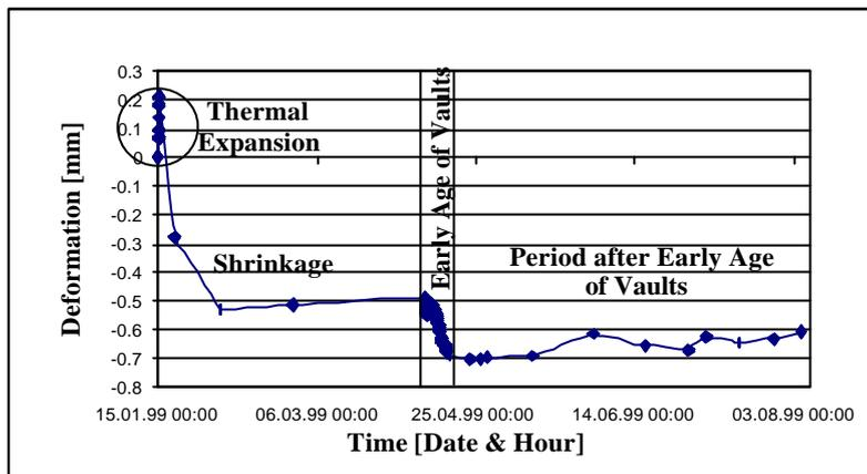
Figure 4. Deformation history of the foundation measured by sensor S-743
