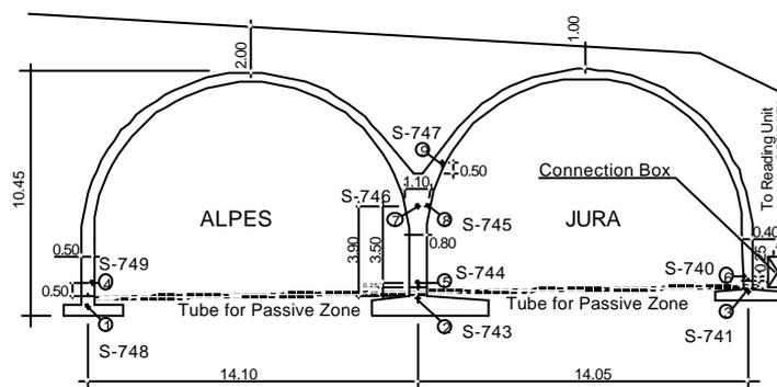
**Figure 3.** Position of sensors in monitored cross-section of cut-and-cover tunnel of Champ Baly
