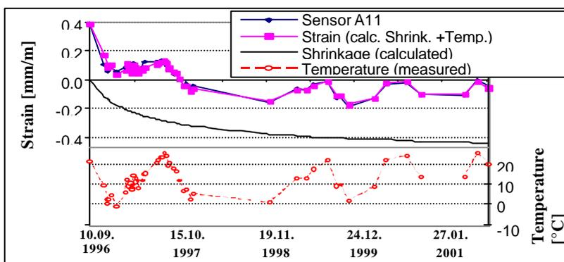
Figure 8. Uncoupling of shrinkage and temperature
