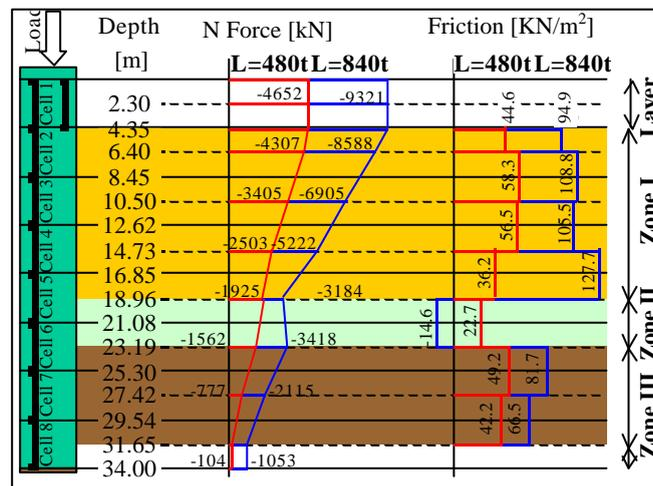
Figure 6. Sensor topology and results obtained by monitoring during the axial compression test
