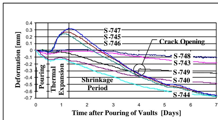
Figure 5. Deformation measurements during the early age of the vaults
