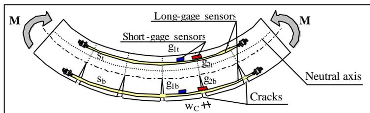
Figure 2. Difference between material and structural monitoring
