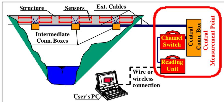
Figure 1. Example of monitoring system installed on structure (SOFO)
