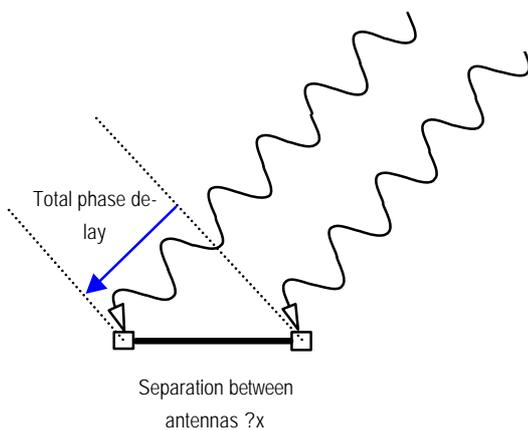
Figure 1. Differential carrier phase measurement principle
