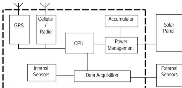
Figure 3. Measurement station block diagram
