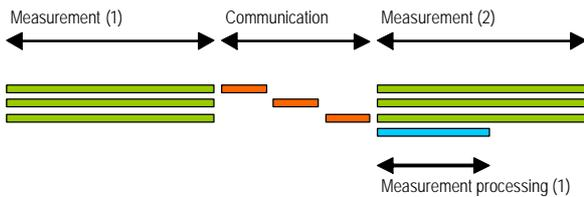
Figure 4. Operating sequence of Measurement stations and Control Center
