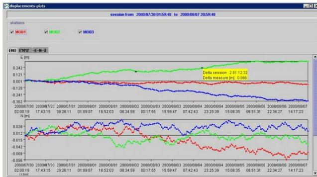
Figure 5. Movements in three dimensions are plotted on the movement screen
