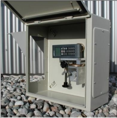
Figure 4: Integrated laser distance meter
