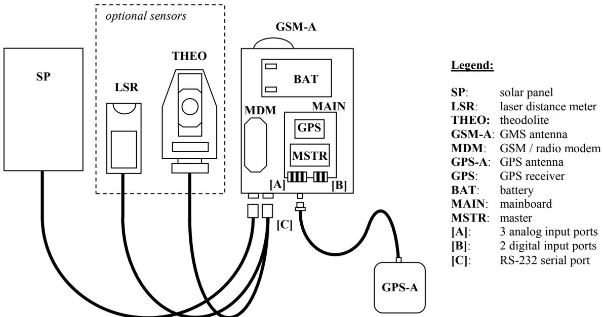
Figure 3: Sensor unit block diagram
